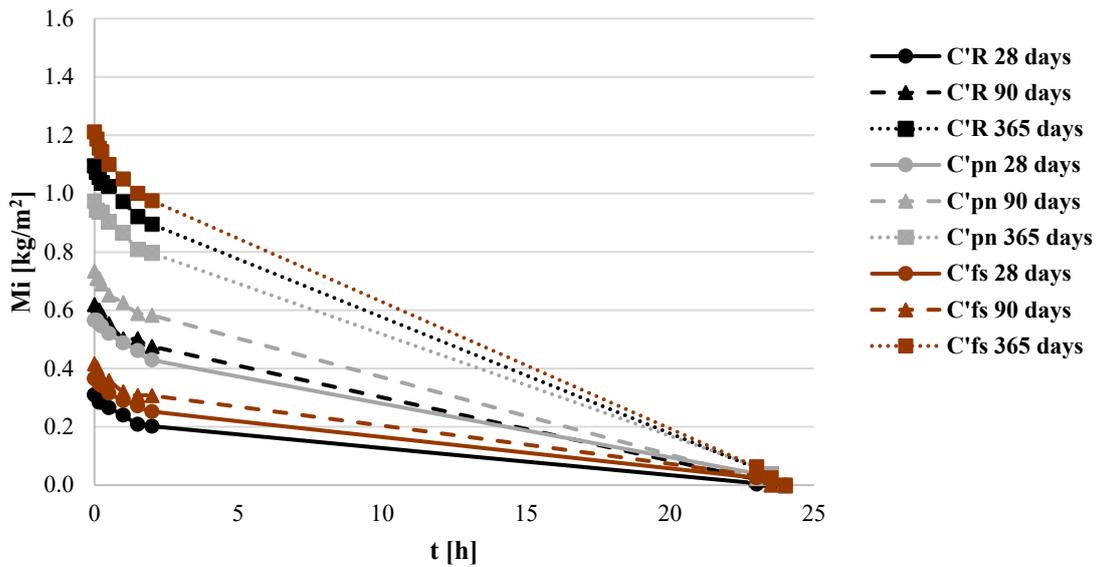
Figure 7. Drying curves of the produced mortars after 28, 90 and 365 hardening days.
