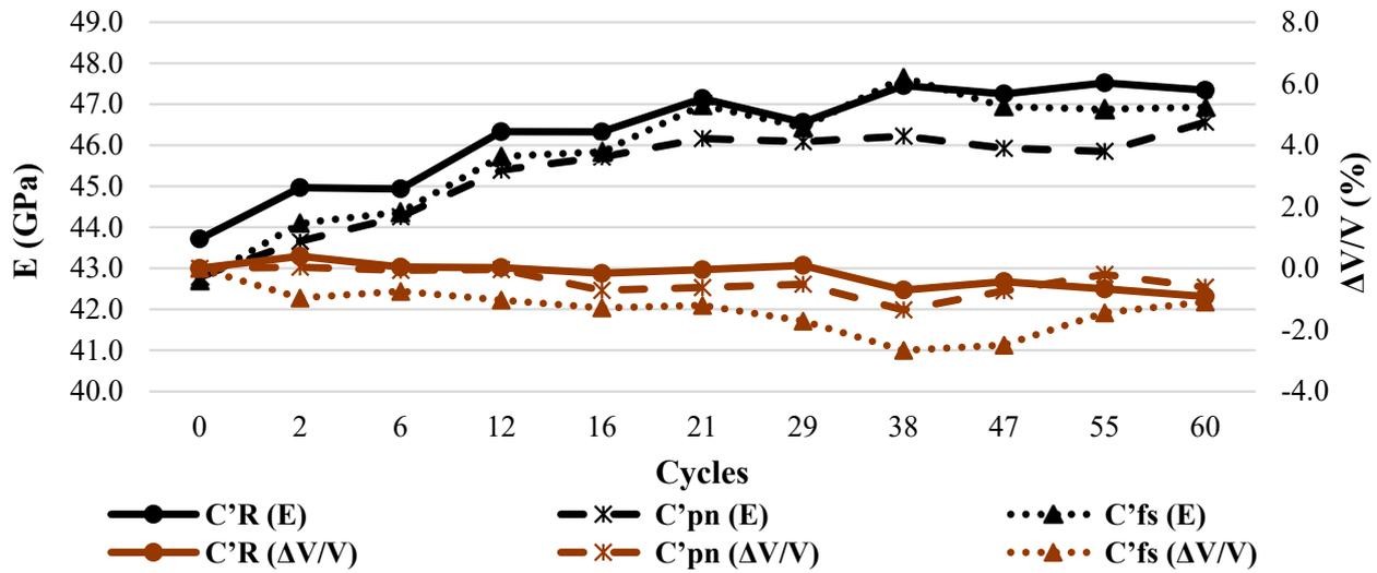
Figure 9. Dynamic moduli of elasticity (E) and volume deformations ( $\Delta V/V$ ) of the produced mortars during freeze–thaw cycles.
