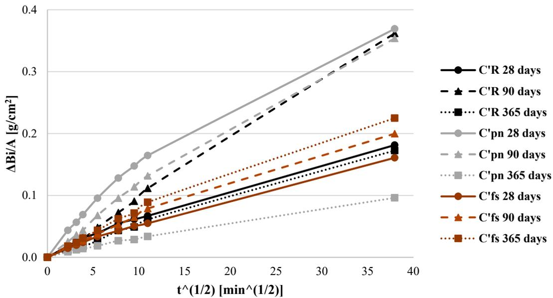
Figure 5. Capillary absorption of the cement mortars at the ages of 28, 90 and 365 days.
