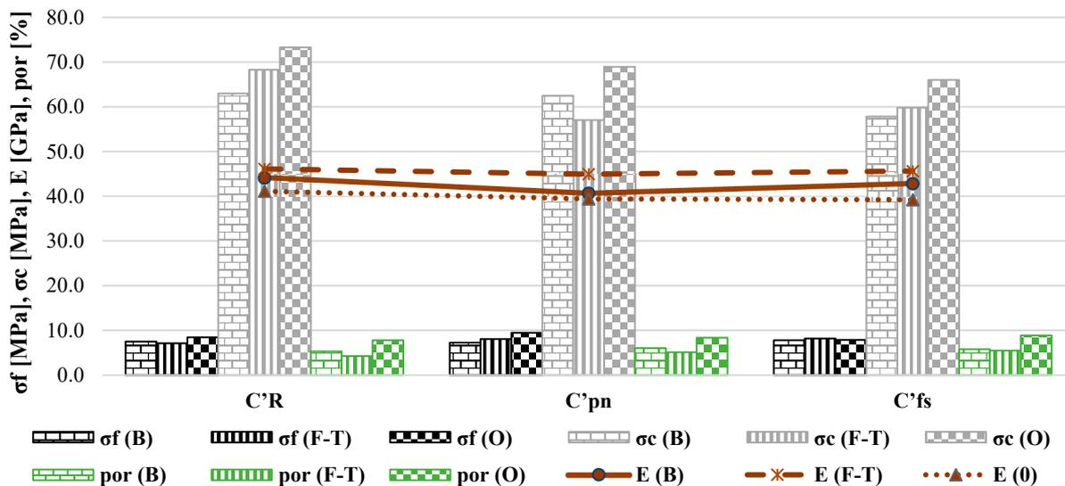
**Figure 11.** Flexural strengths ( $\sigma_f$ ), compressive strengths ( $\sigma_c$ ), dynamic moduli of elasticity (E) and porosity (por) of the produced mortars before the start of cycles (B) and at the end of the freeze–thaw cycles (F–T) or outdoor exposure (O).
