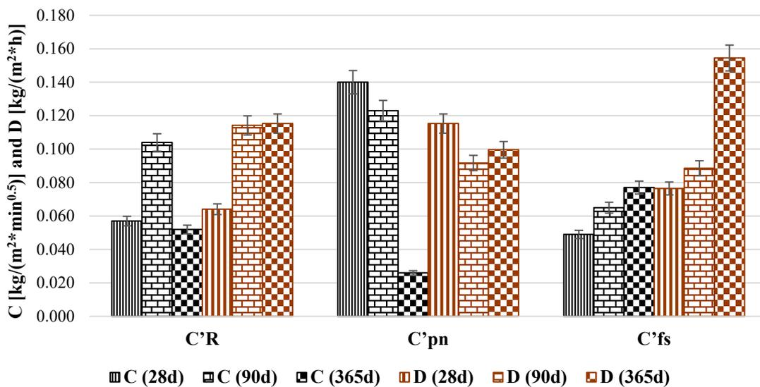
Figure 6. Capillary water absorption coefficient (C) and drying rate for the first 24 h of drying (D) of the cement mortars at the ages of 28, 90 and 365 days (28 d, 90 d and 365 d).
