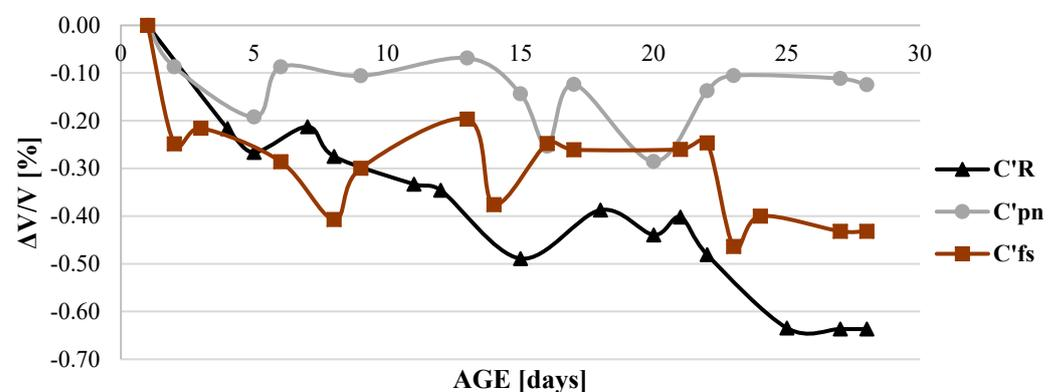
**Figure 4.** Volume deformations of the produced mortars (C'R: reference/unreinforced mixture, C'pn: reinforced mixture with black pine fibres, C'fs: reinforced mixture with beech fibres).
