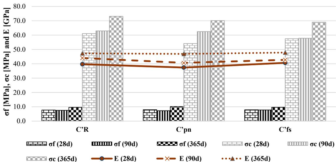
Figure 8. Flexural strengths ( $\sigma_f$ ), compressive strengths ( $\sigma_c$ ) and dynamic moduli of elasticity (E) of the produced mortars at the ages of 28, 90 and 365 days (28 d, 90 d and 365 d).
