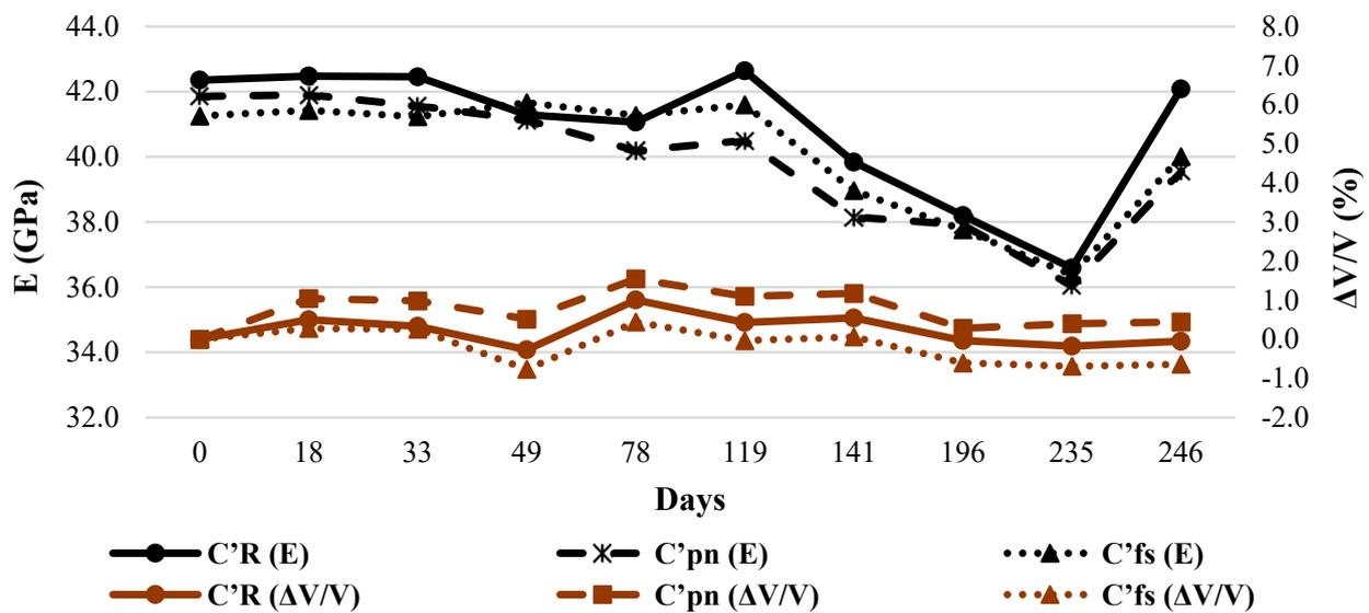
Figure 10. Dynamic moduli of elasticity (E) and volume deformations ( $\Delta V/V$ ) of the produced mortars at days of exposure to outdoor conditions.
