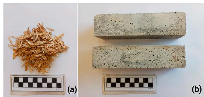
**Figure 3.** Wood fibres of beech species (*Fagus sylvatica* L.) (a) and the respective specimens of wood–cement mortars prepared for the static bending strength test (b).
