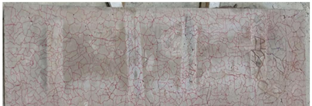
Figure 7. Crack developed by thermal shock.
