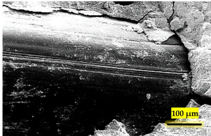
**Figure 13.** SEM image of the surface of BFP in S50-B2.5 subjected to the salt–frost exposure after flexural loading displaying no signs of pellet degradation [49].
