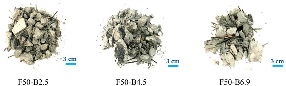
**Figure 7.** Failure modes for the fly-ash-based NFRCC after impact load test [49].
