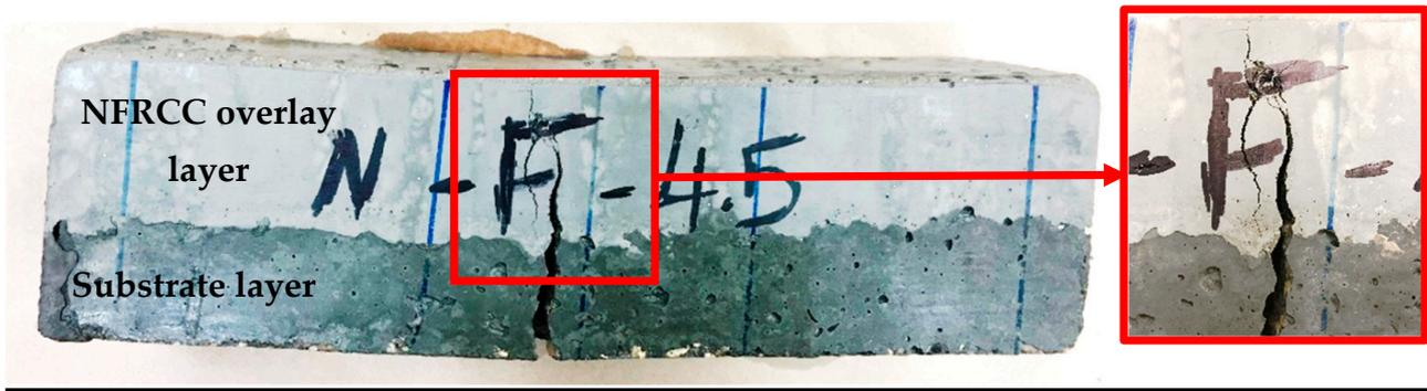
Figure 14. F50-B4.5 overlay sample after flexural test [49].
