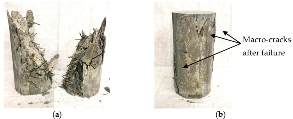
**Figure 20.** Failure mode of specimens after the compressive strength test at 56 days: (a) S50-B2.5 and (b) S50-B2.5 with PVAF [70].
