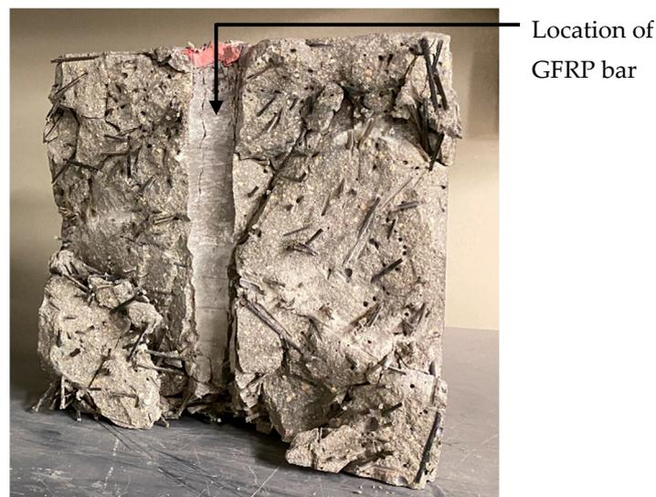
**Figure 18.** BFP distribution in the specimen with 4.5% BFPs [60].
