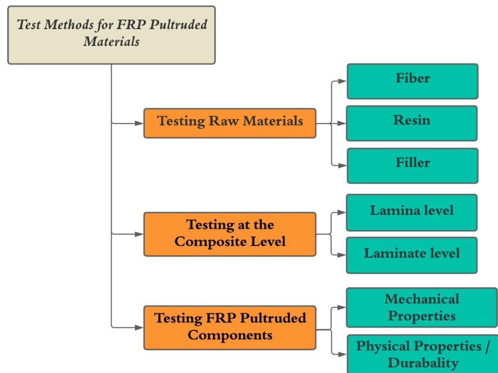
**Figure 3.** Test methods for FRP pultruded materials.
