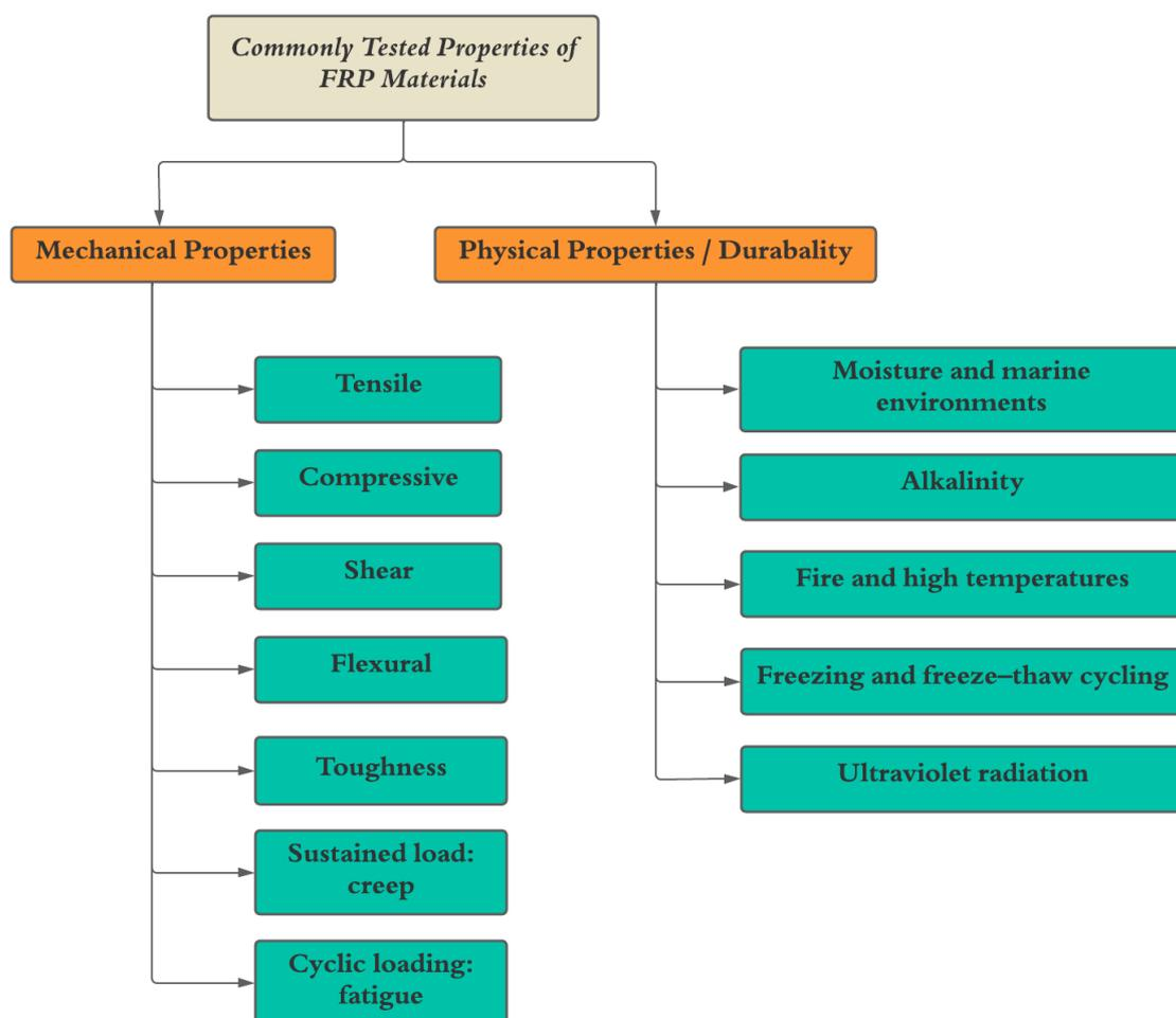
**Figure 4.** Commonly tested properties of FRP materials.
