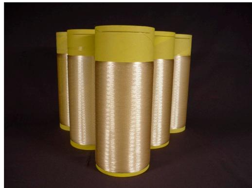
**Figure 4.** HP spun filament fibers.
