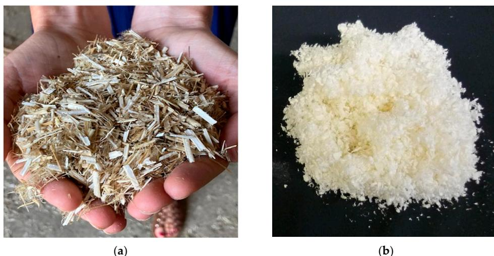
**Figure 1.** (a) Shredded hemp after processing in the decortication line; (b) hemp pulp (HP) as received.
