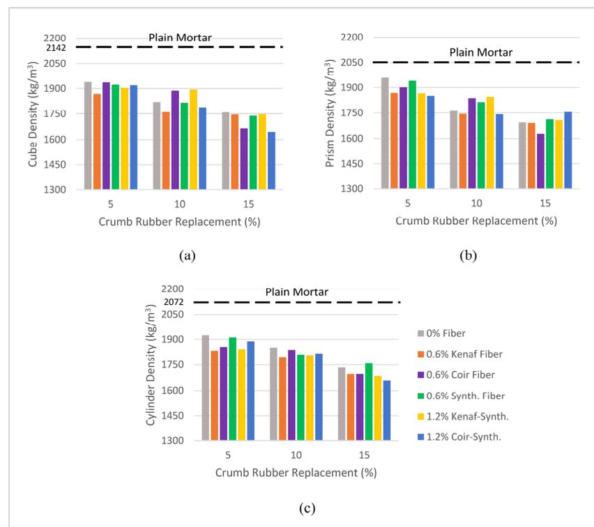
**Figure 5.** The density of CRM specimens. (a) Total cube density. (b) Total prism density. (c) Total cylinder density.
