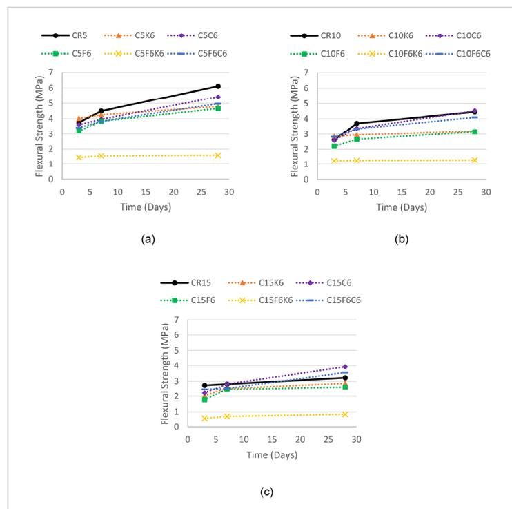
**Figure 7.** Flexural strength comparison for fiber-reinforced CRM at 3, 7, and 28 days. (a) 5% CR replacement. (b) 10% CR replacement. (c) 15% CR replacement.
