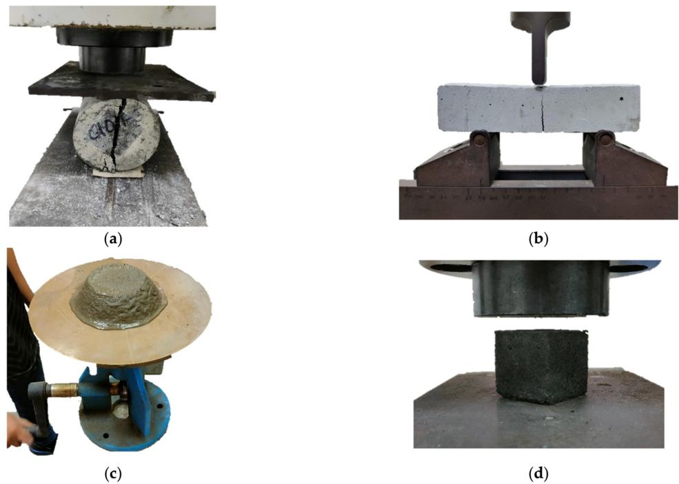
**Figure 3.** Test setup for experimental testing. (a) Indirect tensile strength test. (b) Flexural strength test. (c) Flowability test. (d) Compressive strength test.
