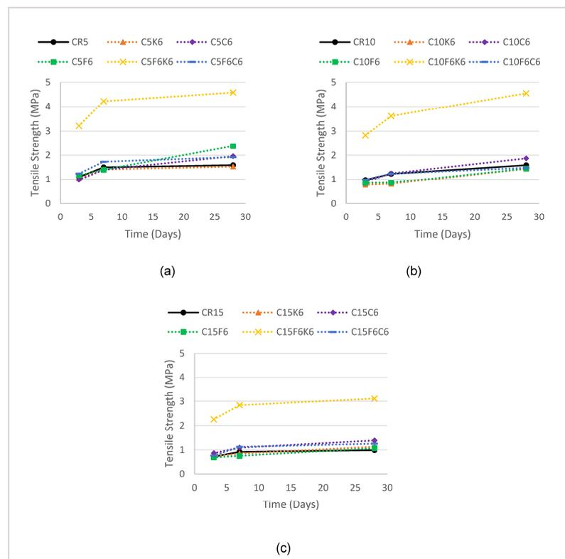
**Figure 8.** Tensile strength comparison for fiber-reinforced CRM at 3, 7, and 28 days. (a) 5% CR replacement. (b) 10% CR replacement. (c) 15% CR replacement.
