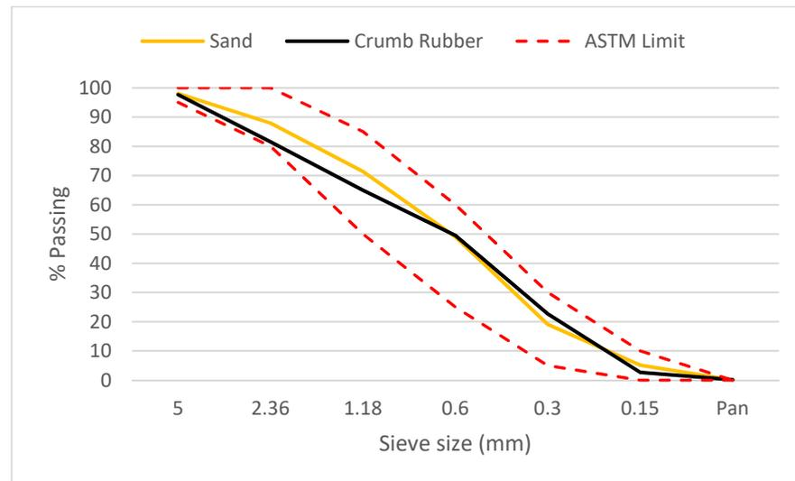
Figure 1. Grading curves for sand and crumb rubber aggregates.
