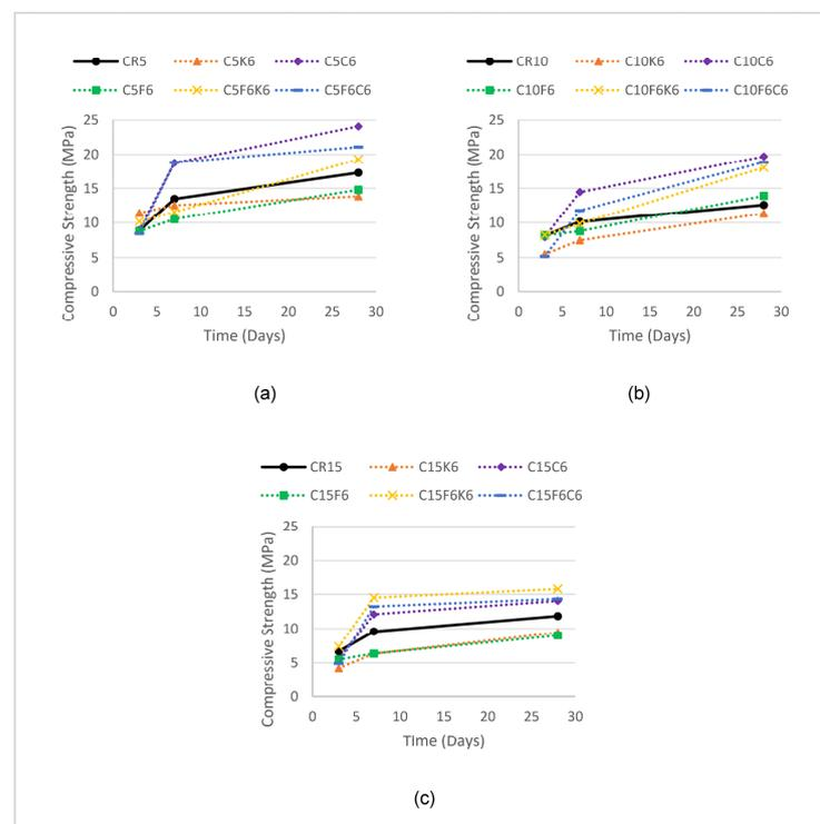
**Figure 6.** Compressive strength comparison for fiber-reinforced CRM at 3, 7, and 28 days. (a) 5% CR replacement. (b) 10% CR replacement. (c) 15% CR replacement.
