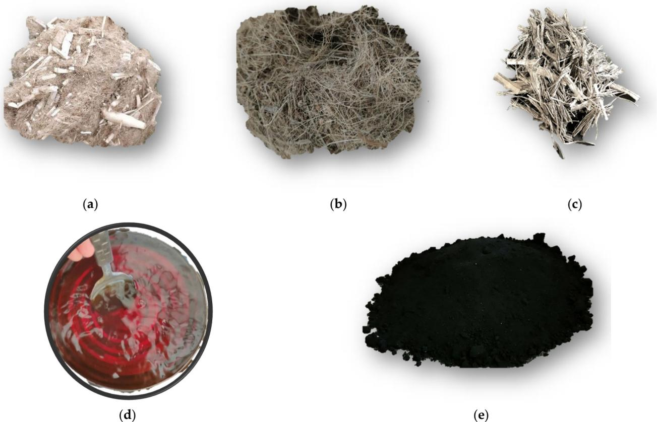
Figure 2. Raw materials used in this study. (a) Kenaf fibers. (b) Coconut fibers. (c) Synthetic fibers. (d) Chemical admixture. (e) Crumb rubber aggregate.
