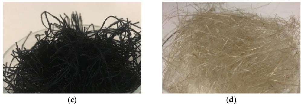
**Figure 1.** Fibre's waste used: (a) wool fibres, (b) coir fibres, (c) textile-acrylic fibres and (d) flax fibres.
