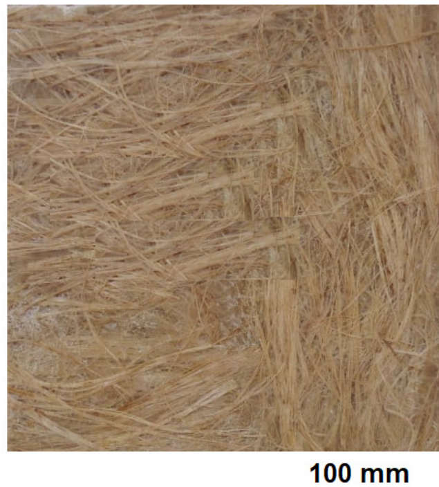
Figure 2. Random banana–kenaf reinforcement for resin impregnation.
