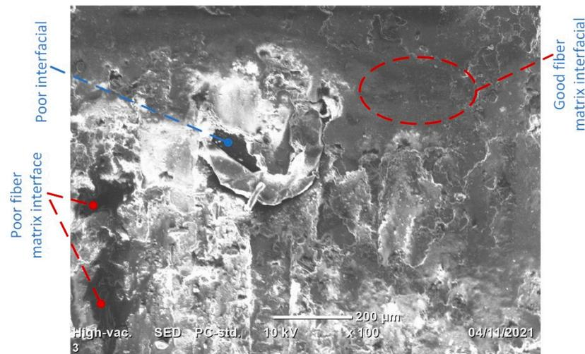
**Figure 9.** SEM image of 0/100 of enset-sisal hybrid composite.
