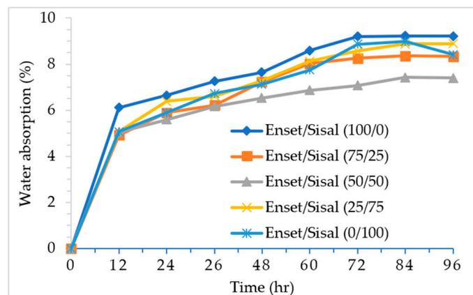
**Figure 7.** Moisture absorption test result of hybrid enset–sisal hybrid composites.
