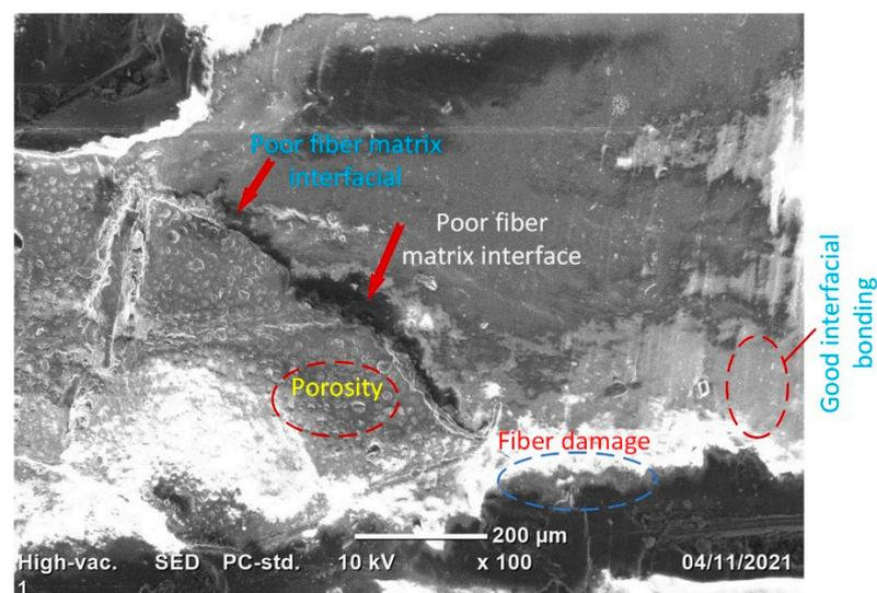
**Figure 8.** SEM image of 100/0 of enset–sisal hybrid composite.
