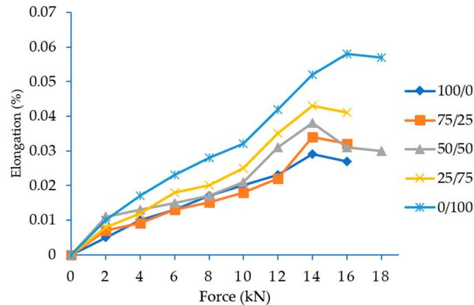
**Figure 4.** Force–elongation diagram for (tensile) for enset sisal hybrid composite.
