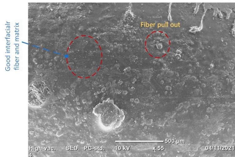
**Figure 10.** SEM image of 50/50 of enset-sisal hybrid composite.
