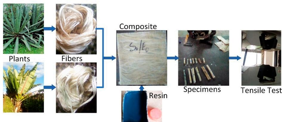
**Figure 1.** The composite fabrication process flow diagram.
