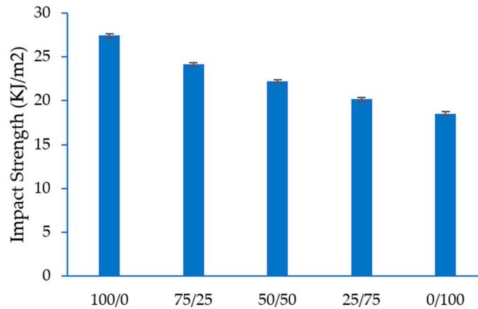
**Figure 6.** Impact Strength test result of enset–sisal hybrid composites.
