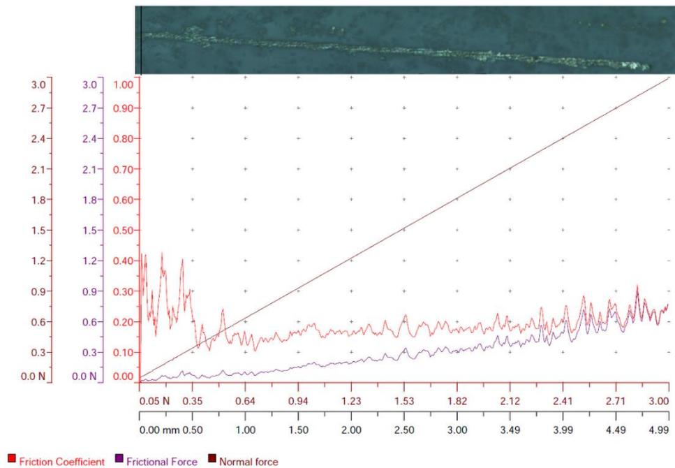
**Figure 8.** The friction force which occurred under the loads applied during Scratch testing of the coatings formed at 150 V and a 1 min period, and the variation of the friction coefficients.
