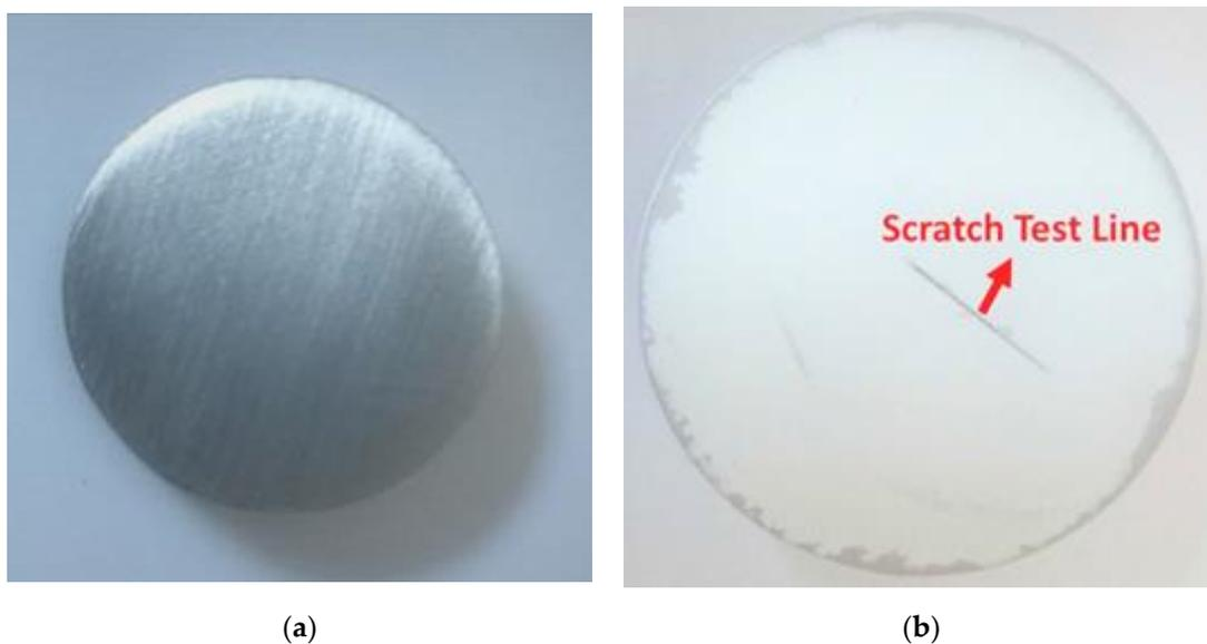
Figure 1. TiAl7Nb alloys: (a) pre-coating and (b) post-coating images.
