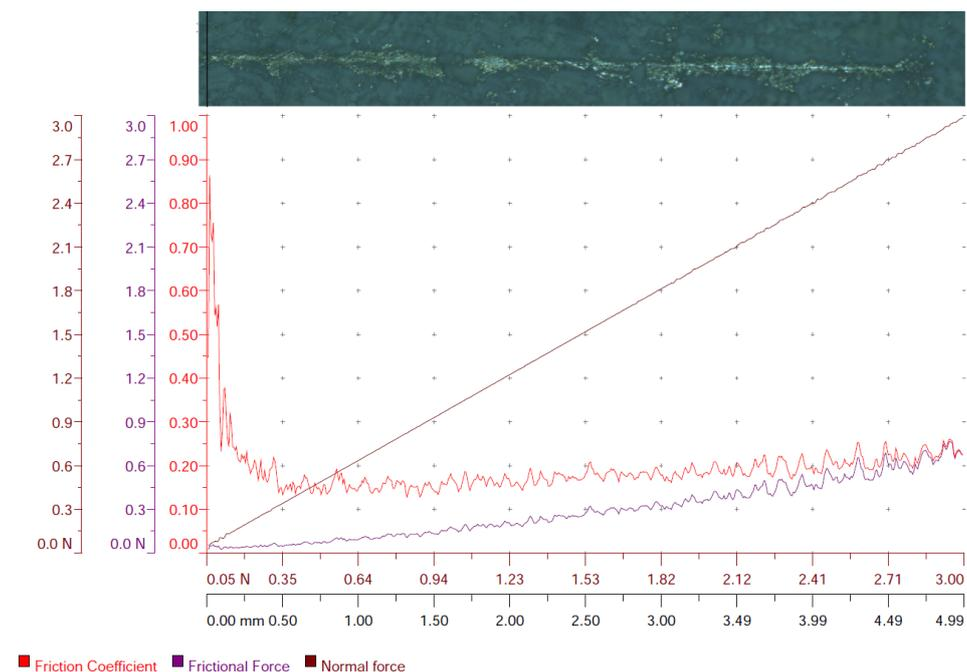
**Figure 9.** The friction force which occurred under the loads applied during Scratch testing of the coatings formed at 200 V and a 1 min period, and the variation of the friction coefficients.
