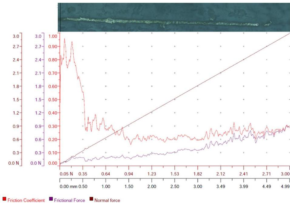
**Figure 7.** The friction force which occurred under the loads applied during Scratch testing of the coatings formed at 100 V and a 1 min period, and the variation of the friction coefficients.
