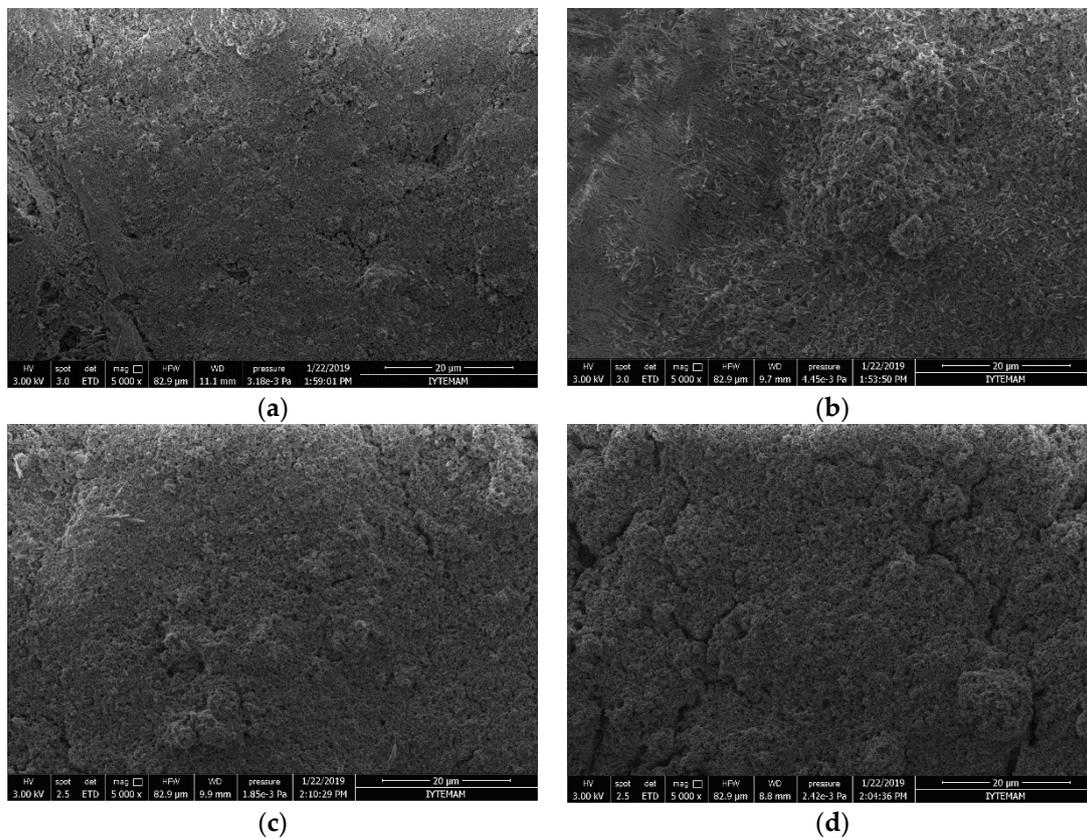
**Figure 3.** SEM images of hydroxyapatite (HA)-coated Ti6Al7Nb alloys (5000 $\times$ ): (a) 50 V/60 s, (b) 100 V/60 s, (c) 150 V/60 s, (d) 200 V/60 s.
