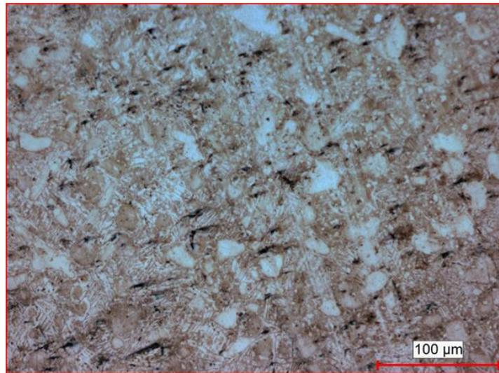
**Figure 2.** Optical microscope image of the Ti6Al7Nb alloy surface prior to coating.
