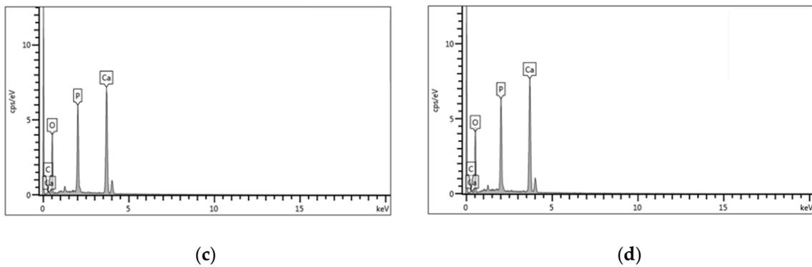
**Figure 4.** The EDS results of HA-coated Ti6Al7Nb alloys: (a) 50 V/60 s, (b) 100 V/60 s, (c) 150 V/60 s, (d) 200 V/60 s.
