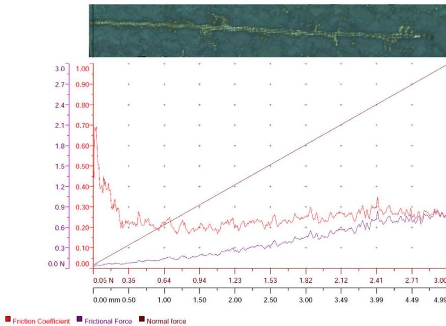
**Figure 6.** The friction force which occurred under the loads applied during Scratch testing of the coatings formed at 50 V and a 1 min period, and the variation of the friction coefficients.
