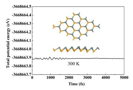
**Figure S1.** Total potential energy of pristine monolayer SnSe at 300 K within 5 ps during the first-principles molecular dynamics (MD) simulation.
