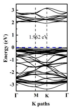
**Figure S3.** Band structure of the monolayered  $\beta$ -SnSe with the H<sub>2</sub>O molecules.
