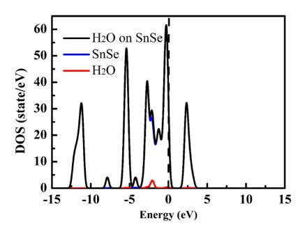
**Figure S4.** Total DOSs of the H<sub>2</sub>O on SnSe (black curve), the projected DOS of SnSe (red curve), and the adsorbate molecules (blue curve) for H<sub>2</sub>O on SnSe monolayer. The *E*<sup>*t*</sup> is set to zero, as illustrated by black dotted line.
