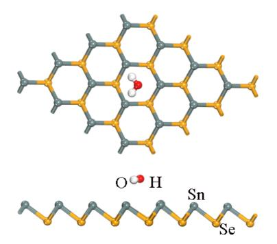
Figure S2. The most stable site of structural optimizations for H<sub>2</sub>O on  $\beta$ -SnSe layer is presented.
