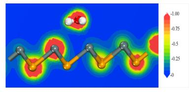
Figure S5. The slice of charge densities for the  $\beta$ -SnSe monolayer with the H<sub>2</sub>O molecule. The value of electron densities ranges between 0 and 1.00 e/Å<sup>3</sup>.
