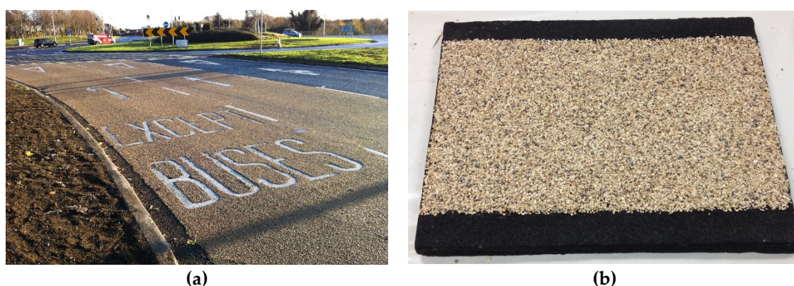
Figure 1. (a) Newly laid HFS system in Ireland; (b) cold applied HFS specimen used in Experiment 1.
