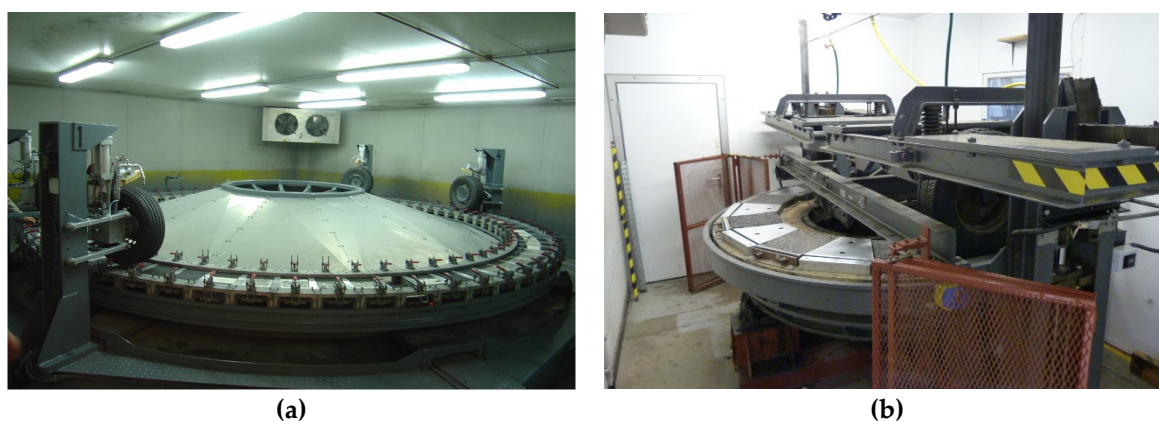
Figure 2. (a) The wear simulator turntable located at Aetec Laboratories, Madrid; (b) the road test machine located at Ulster University.
