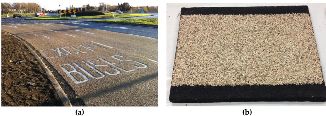
**Figure 1.** (a) Newly laid HFS system in Ireland; (b) cold applied HFS specimen used in Experiment 1.
