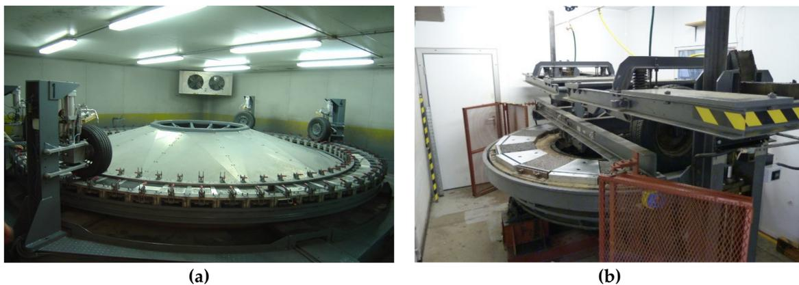
**Figure 2.** (a) The wear simulator turntable located at Aetec Laboratories, Madrid; (b) the road test machine located at Ulster University.
