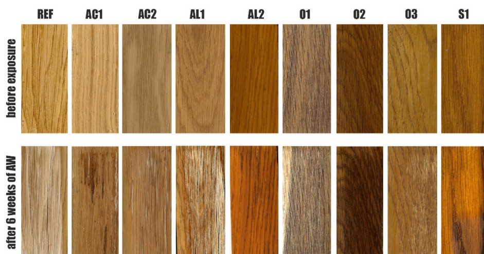
Figure 5. Visual evaluation of tested coatings before and after 6 weeks of AW exposure.
