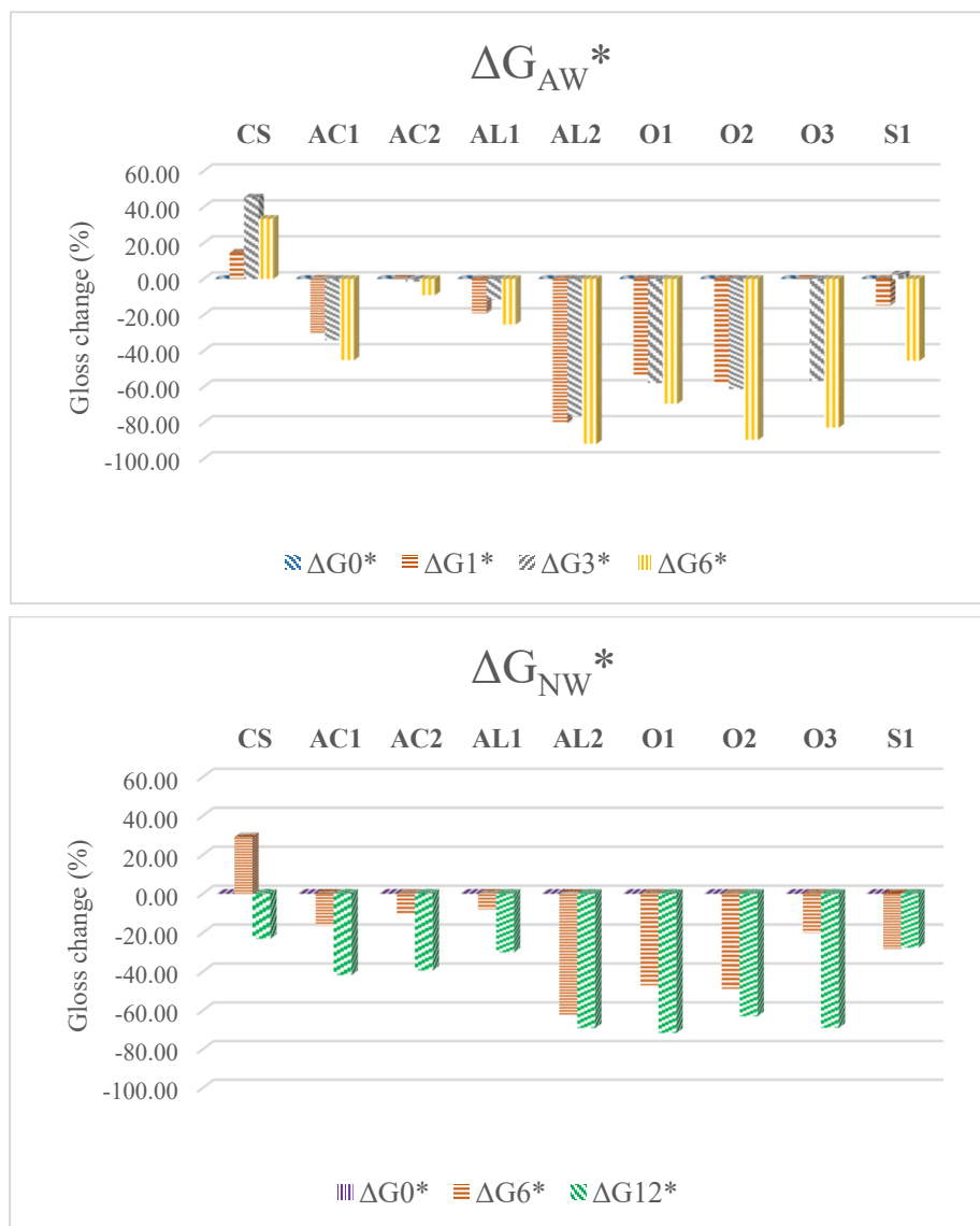
Figure 3. Gloss difference ( \Delta G^* ) of tested coating systems during artificial and natural weathering (CS means control sample).
