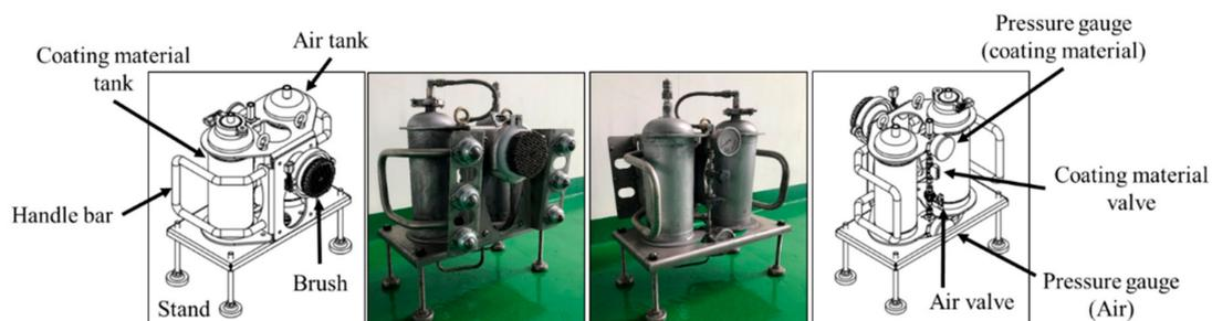
**Figure 2.** Front and rear parts of EQ3.
