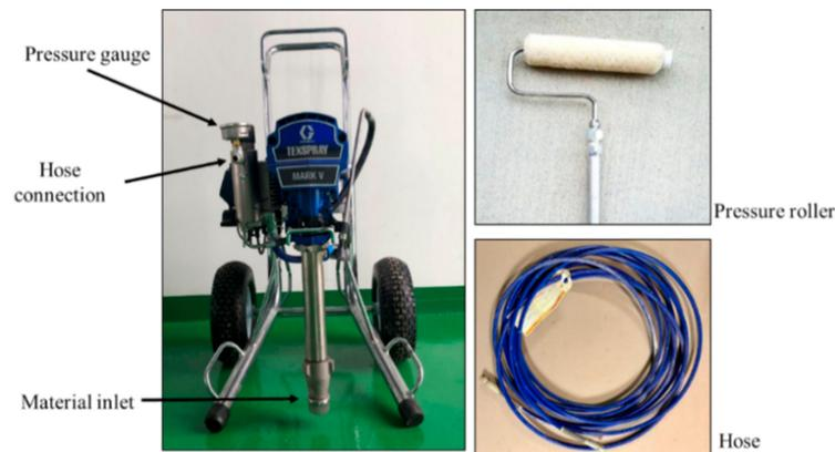
**Figure 1.** Selected equipment (EQ2) that uses an airless pump.
