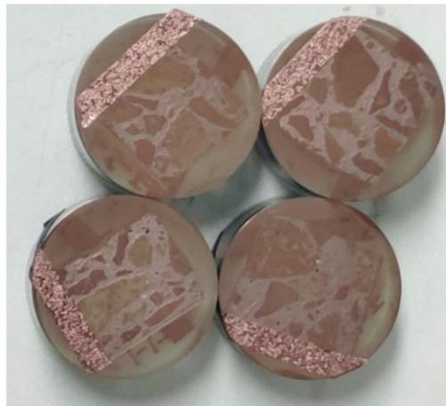
**Figure 9.** Prepared samples for SEM analysis.
