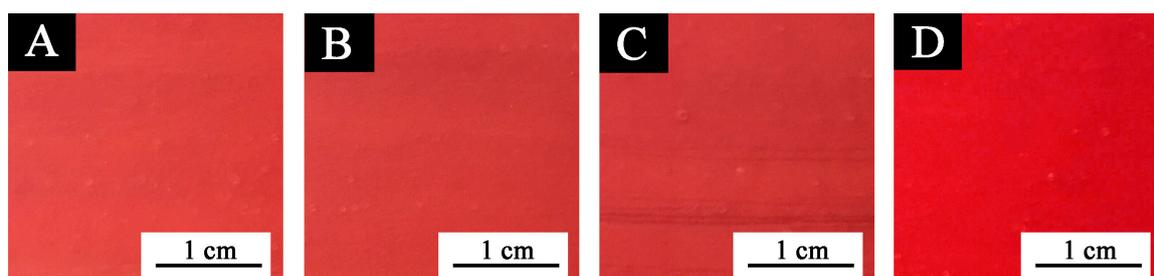
**Figure 2.** Images of coatings with 10% thermochromic pigment powder after liquid resistance test: (A) NaCl, (B) detergent, (C) ethanol, and (D) red ink.
