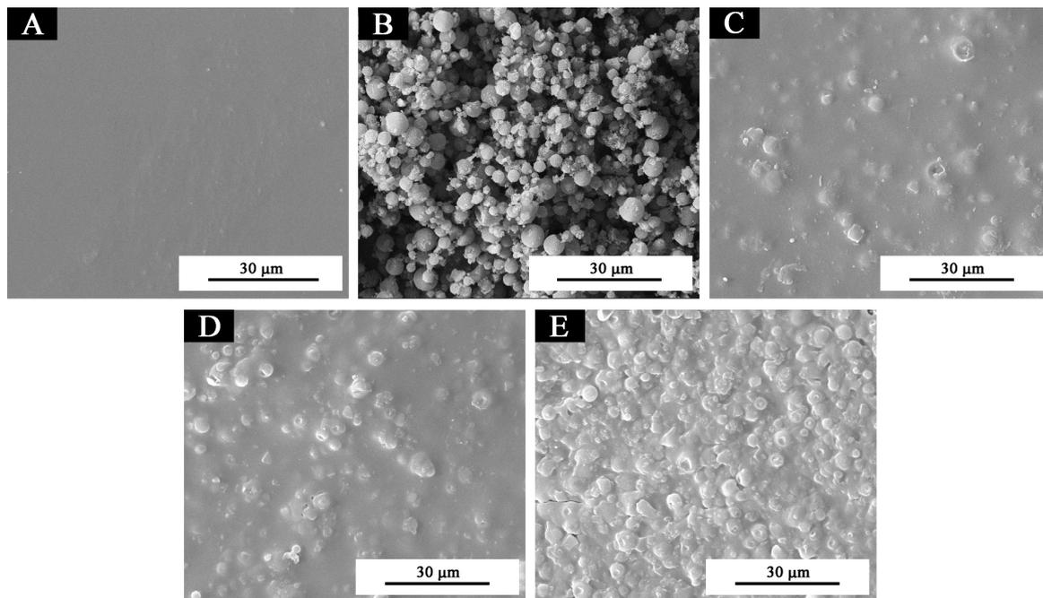
**Figure 3.** SEM of different concentrations of thermochromic pigment powder in the waterborne primer: (A) pure waterborne primer film; (B) thermochromic pigment powder; (C–E) 5%, 10% and 30% thermochromic pigment powder in the waterborne primer, respectively.
