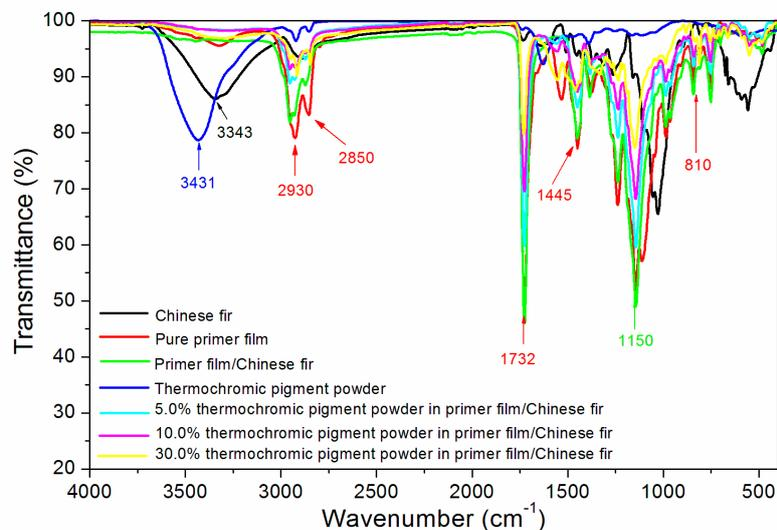
**Figure 4.** FTIR of different concentrations of thermochromic pigment powder in the waterborne primer film.
