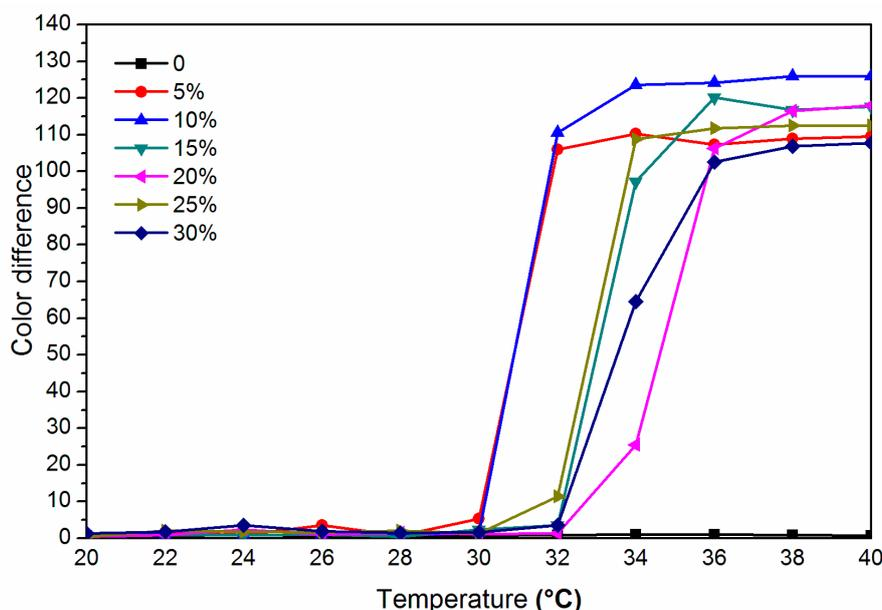
**Figure 1.** The effect of concentration of thermochromic pigment powder on color difference of waterborne primer film from 18 to 40 °C.
