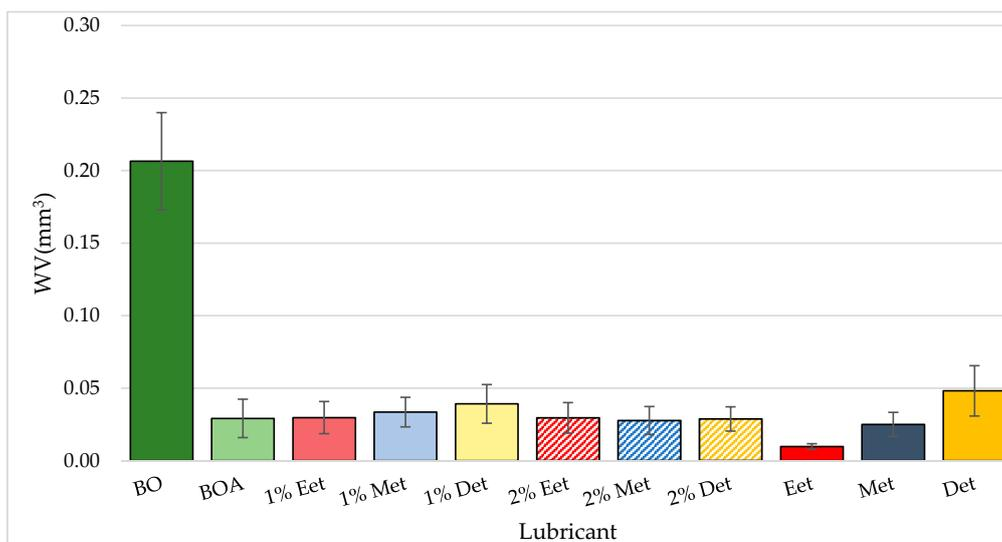
Figure 6. Average values of the wear volume of steel disks after tests lubricated with BO, BOA, neat PILs, and PIL blends 1 wt.% Eet + BO, 1 wt.% Met + BO, and 1 wt.% Det + BO.
