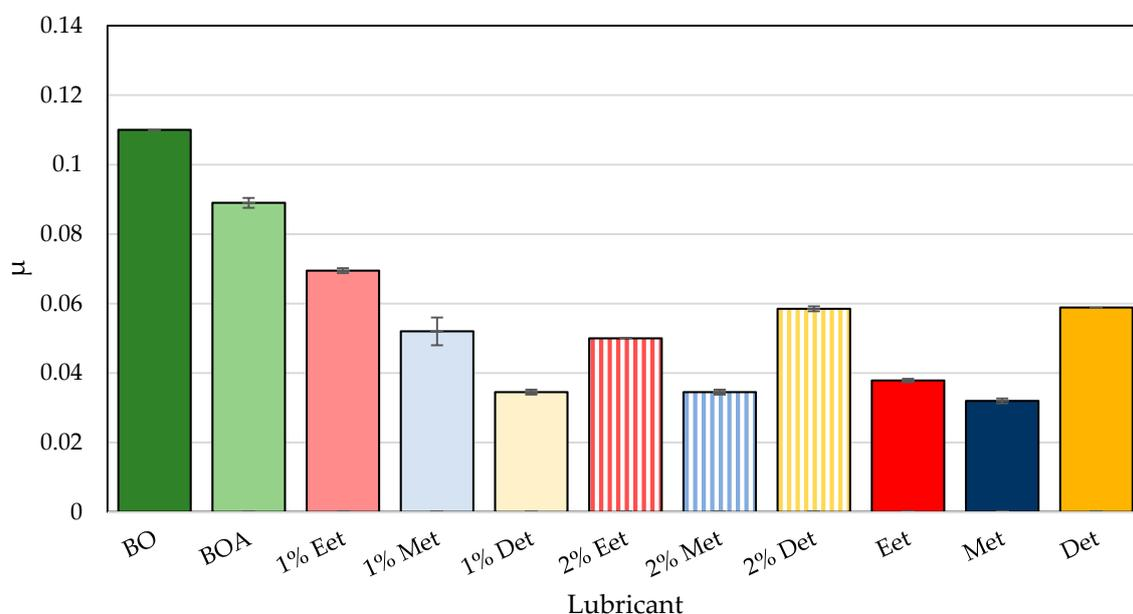
**Figure 4.** Average friction coefficients of steel–steel contact after tests lubricated with BO, BOA, neat PILs, and PIL blends 1 wt.% Eet + BO, 1 wt.% Met + BO, and 1 wt.% Det + BO.
