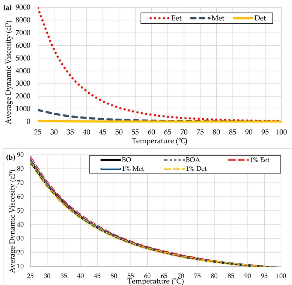
**Figure 2.** Average dynamic viscosity as a function of temperature for (a) the neat PILs and (b) biodegradable base (BO), BIO TELEX 46 (BOA), and 1 wt.% PIL blends.
