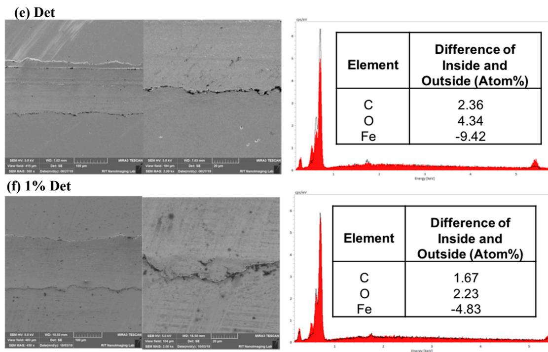
**Figure 9.** SEM images of worn surfaces and energy-dispersive X-ray (EDX) spectrum results of the inside and outside wear tracks for different lubricant conditions: (a) BO, (b) BOA, (c) Eet, (d) Met, (e) Det, and (f) 1 wt.% Det + BO.
