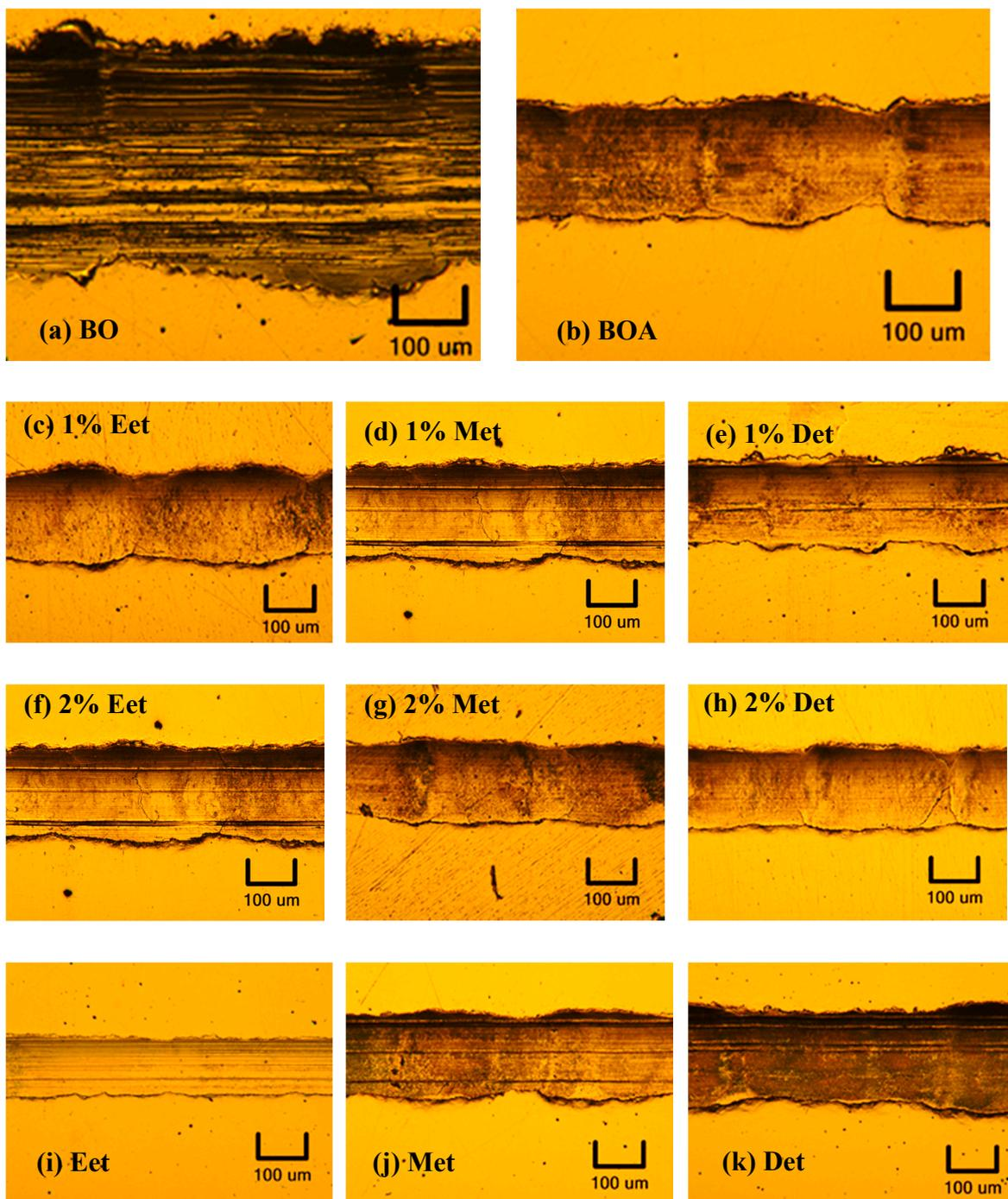
**Figure 7.** Optical images of worn surfaces on steel surfaces after tests lubricated with (a) BO, (b) BOA, (c) 1 wt.% Eet + BO, (d) 1 wt.% Met + BO, (e) 1 wt.% Det + BO, (f) 2 wt.% Eet + BO, (g) 2 wt.% Met + BO, (h) 2 wt.% Det + BO, (i) Eet, (j) Met, and (k) Det.
