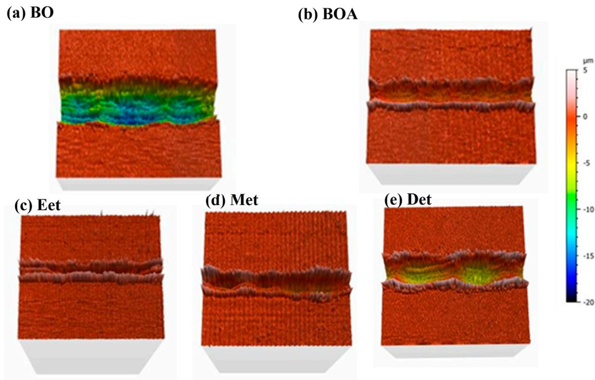
**Figure 8.** Three-dimensional (3D) surface profiles on steel surfaces after tests lubricated with (a) BO, (b) BOA, (c) Eet, (d) Met, and (e) Det.
