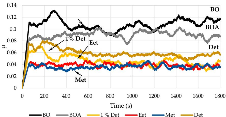
Figure 5. Friction vs. time curves of BO, BOA, 1 wt.% Det + BO, Eet, Met, and Det.
