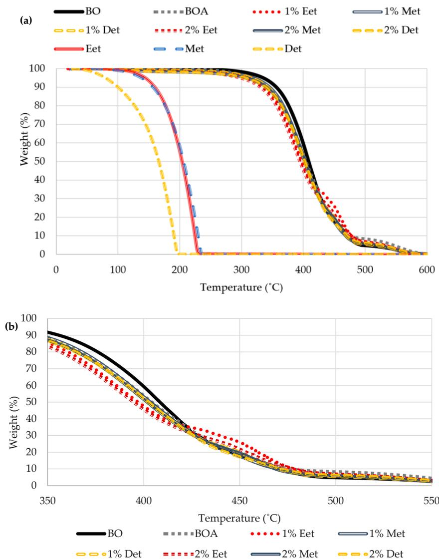
**Figure 3.** (a) Experimental TGA for BO, BOA, neat PILs, and PIL blends, (b) detail of the thermalgravimetric behavior of the lubricants from 350 to 550 °C.
