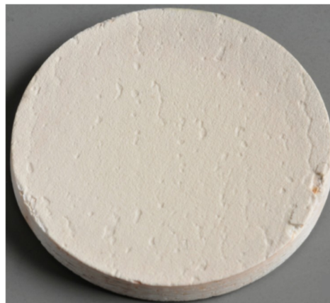
Figure 9. Photograph of VLPPS \text{YAlO}_3 coating on FW12 after 1010 cycles of burner rig testing.
