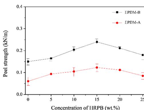
**Figure 3.** Peel strengths of CPP/Al foil laminates vs HRPB (wt.%) content of the adhesives, which were laminated with EPDM-B (■) or EPDM-A (●). The failures occurred at interfaces of adhesives and Al foils regardless of concentration of HRPB.
