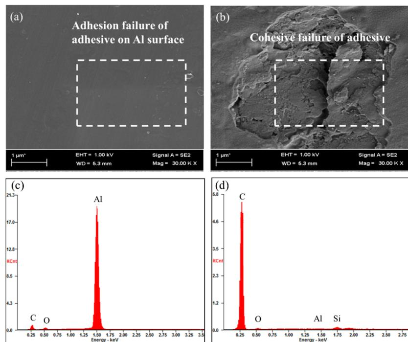
**Figure 10.** SEM images and EDX results of the Al surfaces of CPP/EPDM-B-15/Al foil and CPP/EPDM-B-15/APTES-treated Al foil laminates after peel test. The peel test was conducted after tempering of the laminates at 80 °C for 1 day: (a) Al surface of CPP/EPDM-B-15/Al foil; (b) APTES-treated Al foil surface of CPP/EPDM-B-15/APTES-treated Al foil; (c,d) EDX results in the area assigned with white dotted line in (a) and (b) respectively.
