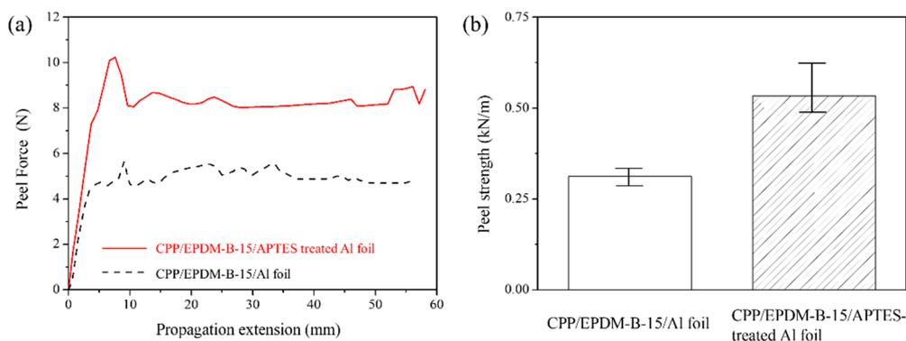
**Figure 9.** Results of the 180° peel test after tempering at 80 °C for 1 day: (a) typical peel force (N) vs. propagation extension (mm) of CPP/EPDM-B-15/APTES-treated Al foil and CPP/EPDM-B-15/Al foil, (b) peel strength (kN/m) of CPP/EPDM-B-15/APTES-treated Al foil and CPP/EPDM-B-15/Al foil.
