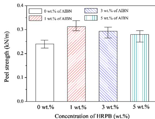
**Figure 5.** Effect of radical initiator content on the peel strength of EPDM-B-15-based CPP/Al foil laminates. The failure occurred at interfaces between EPDM-B-15 and Al foil regardless of concentration of AIBN.
