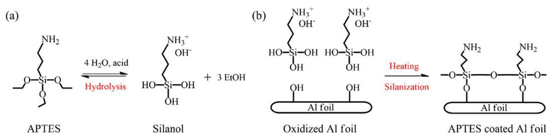
**Figure 6.** Mechanism for the surface treatment of Al foil with APTES: (a) hydrolysis of APTES in acidic condition; (b) silanization between oxidized Al foil and silanol.
