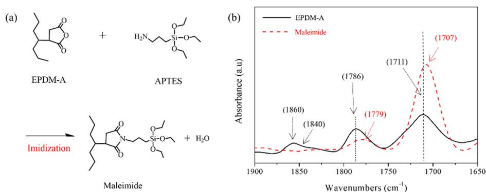
**Figure 8.** Schematic for the imidization of the MAH groups of EPDM-A and amine groups of APTES (a) and FT-IR spectra of EPDM-A (black) and maleimide synthesized from reaction between EPDM-A and APTES (red dot line) (b).
