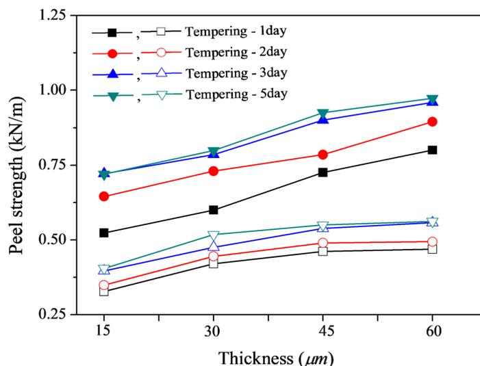
**Figure 11.** Effects of adhesive thickness and tempering time on the adhesive strength of CPP/EPDM-B-15/Al foil (open symbol) and CPP/EPDM-B-15/APTES-treated Al foil (filled symbol).
