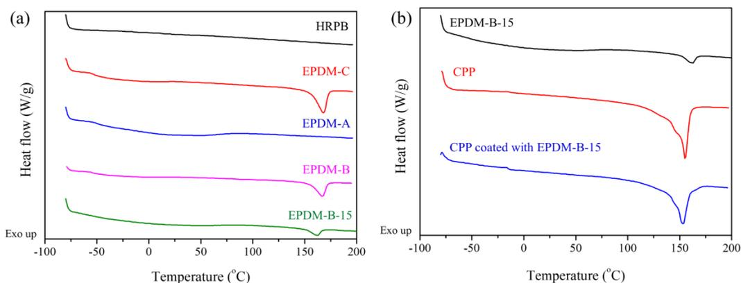
**Figure 4.** DSC thermograms during heating for (a) raw materials and EPDM-B-15 and (b) EPDM-B-15, CPP film and CPP coated with EPDM-B-15.
