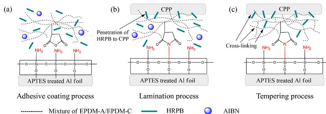
**Figure 2.** Overall scheme for CPP and Al foil adhesion. (a) The prepared adhesive is uniformly coated on the APTES treated Al foil using a bar coater; (b) The EPDM-A/EPDM-C form maleimide groups via imidization with the  $\text{-NH}_2$  groups of APTES and wet onto CPP during lamination at 110 °C; (c) The mixture of EPDM-A/EPDM-C and HRPB form a cross-linked structure with CPP via radical polymerization during tempering.
