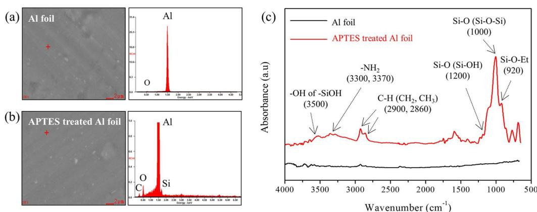
**Figure 7.** SEM images and EDX data of Al foil (a), APTES-treated Al foil (b) and FT-IR spectra of Al foil and APTES-treated Al foil (c).
