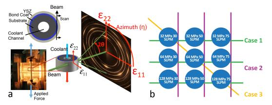
**Figure 1.** (a) view of specimen with attached thermocouple placed in furnace and schematic of experimental methodology with nomenclature of determined strain. (b) Multivariable matrix for Case 1 (constant load, variable flow in standard liters per minute), Case 2 (constant flow, varying mechanical loading), and Case 3 (extrema loading conditions).
