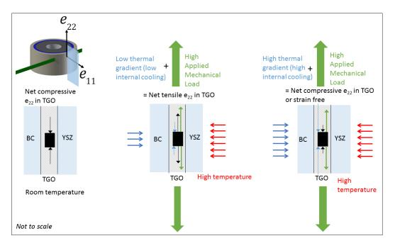
Figure 5. Schematic illustrating the competing effects of applied loads and thermal gradients.
