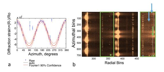
**Figure A2.** Strain analysis and fitting challenges for transformed Debye rings: (**a**) fitting challenges for strain response with bond coat overlap over alumina peak, with representations of in plane (e22) and out of plane (e11) strain data; and (**b**) examination of transformed Debye rings with precipitates obscuring oxide layer ring. Secondary peaks marked in blue interfere with faint TGO peak marked in green.
