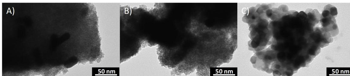
**Figure S2.** TEM micrograph of TiO<sub>2</sub>/AuNRs photocatalysts for different synthesis conditions: TiO<sub>2</sub>/AuNRs 250°C (A); TiO<sub>2</sub>/AuNRs 450°C (B); TiO<sub>2</sub>/AuNRs 650°C (C).
