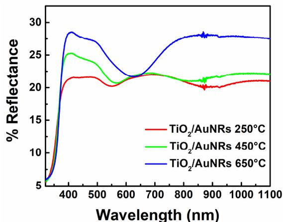
**Figure S3.** Diffuse reflectance spectra (DRS) of TiO<sub>2</sub>/Au NRs nanocomposites deposited onto quartz slides, recorded in absorption mode.
