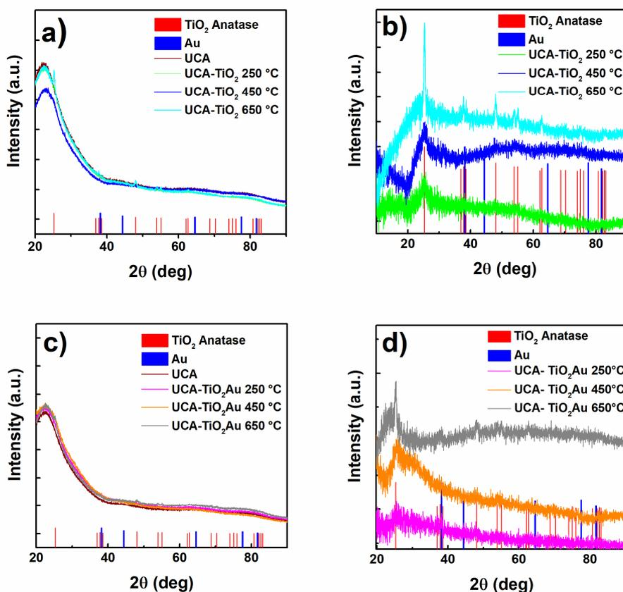
**Figure S4.** XPD patterns of the UCA-TiO<sub>2</sub> and UCA-TiO<sub>2</sub>Au nanocomposites under study. (a,c) Original data of compounds; (b,d) Data corrected by subtracting the contribution of UCA component to enhance the contribution of the TiO<sub>2</sub> nanocrystals and Au NRs.
