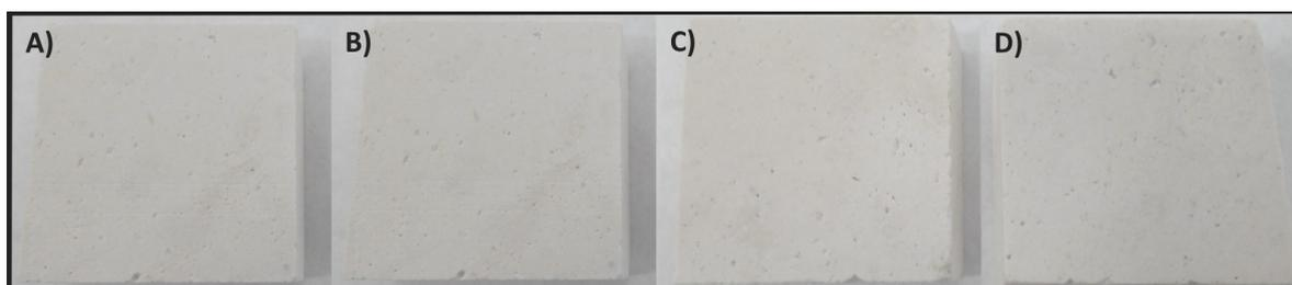
**Figure S5.** Representative pictures of the stones before and after coating: (A) untreated; (B) UCA-TiO<sub>2</sub> P25; (C) UCA-TiO<sub>2</sub> 450 °C; (D) UCA-TiO<sub>2</sub>/Au NRs 450 °C.
