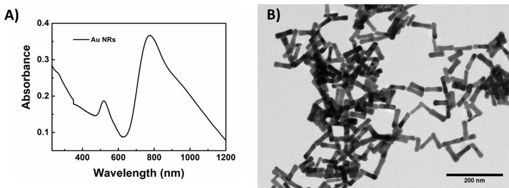
**Figure S1.** (A) UV-Vis absorption spectra of Au NRs solution, after purification in order to remove excess of CTAB; (B) Transmission electron microscopy image of the Au NRs.
