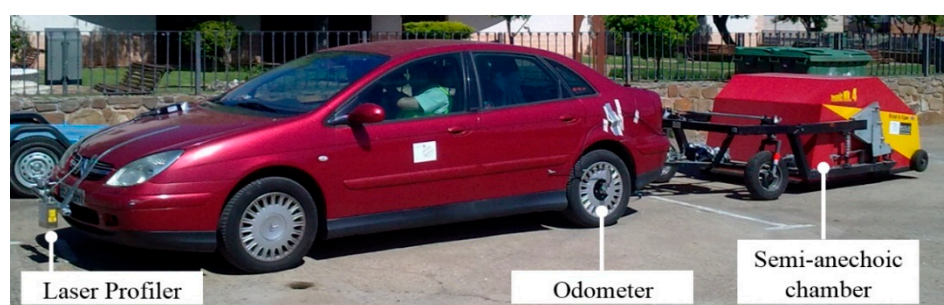
Figure 5. Equipment employed for the simultaneous measure of tire/pavement noise levels and surface profile.
