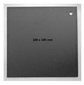
Figure 3. Appearance of a phosphate coating on steel.
