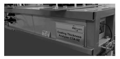
**Figure 2.** XRF gauge CTA-02 analyzer with optoelectronic displacement sensor (at the bottom of the frame on the right).
