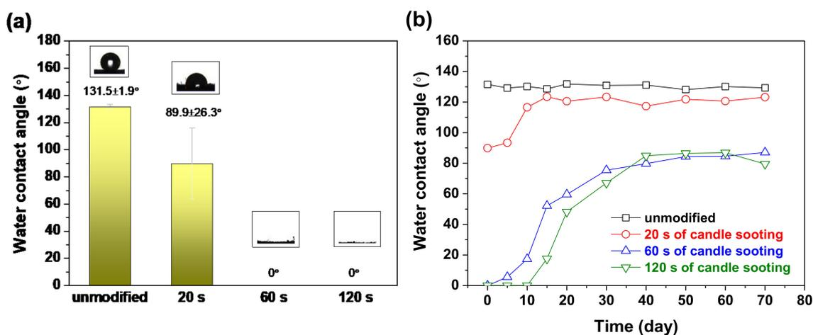
**Figure 4.** (a) Water contact angles of the unmodified carbon cloth and those modified by candle sooting for 20, 60, and 120 s. (b) Water contact angles of the unmodified and candle-soot-modified carbon cloths as a function of the standing time.
