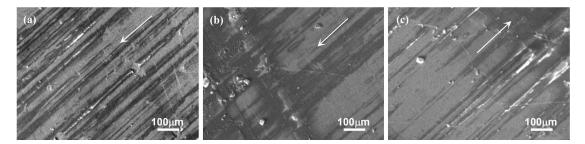
**Figure 4.** SEM images of the transfer layers under different speeds: (a)  $0.1 \text{ m} \cdot \text{s}^{-1}$ ; (b)  $0.4 \text{ m} \cdot \text{s}^{-1}$ ; (c)  $0.8 \text{ m} \cdot \text{s}^{-1}$ .
