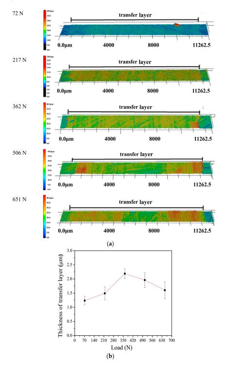
**Figure 9.** (a) The height distribution mappings of transfer layers formed under different loads; (b) The average transfer layer thickness vs. load.
