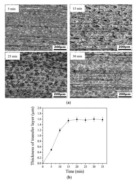
Figure 10. (a) Surface of the counterface at different times; (b) Transfer layer thickness over time.
