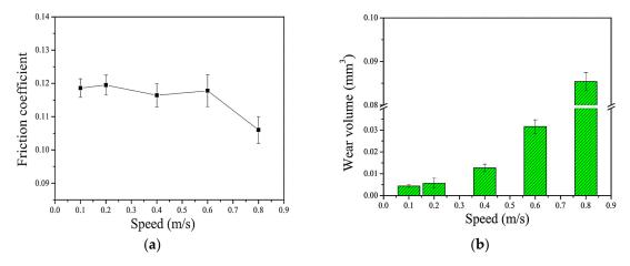
**Figure 3.** The change of friction coefficient and wear under different speeds: (**a**) Friction coefficient vs. speed; (**b**) wear volume vs. speed.
