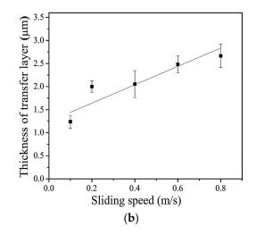
**Figure 6.** (a) The height distribution mappings of transfer layers formed under different sliding speeds; (b) The average transfer layer thickness vs. sliding speed.
