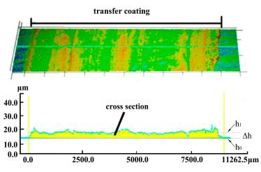
Figure 2. Measuring principle of the transfer layer thickness.
