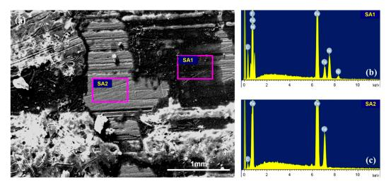
**Figure 5.** SEM and EDS images of the steel surface with and without transfer layers: (**a**) Steel surface with the discontinuous transfer layer; (**b**) EDS image of area SA1; (**c**) EDS image of area SA2.
