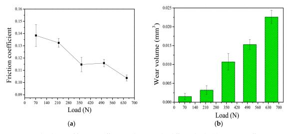
**Figure 7.** The change of friction coefficient and wear under different loads: (**a**) Friction coefficient vs. load; (**b**) wear volume vs. load.
