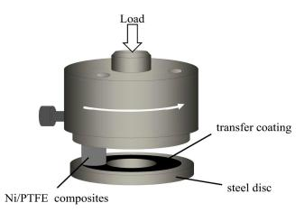
Figure 1. Schematic diagram of the pin-on-disc tribometer.
