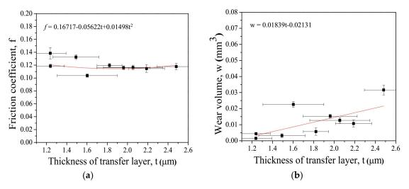
**Figure 11.** Relationships between tribological properties and transfer layer thickness: (**a**) Friction coefficient, (**b**) wear volume.
