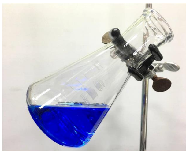
Figure S2. Photograph of the oil collected via the continuous absorption and removal of isooctane from the water surface.
