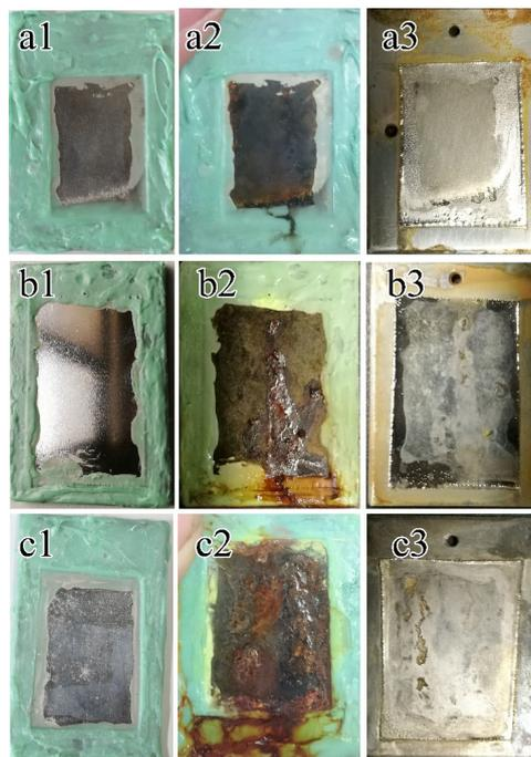
**Figure 9.** Corrosion results of samples deposited under DP. (a1) as deposited; (a2) as deposited after 1000 h test; (a3) as deposited with corrosion product removed; (b1) 300 °C treated; (b2) 300 °C treated after 1000 h test; (b3) 300 °C treated with corrosion product removed; (c1) 400 °C treated; (c2) 400 °C treated after 1000 h test; (c3) 400 °C treated with corrosion product removed.
