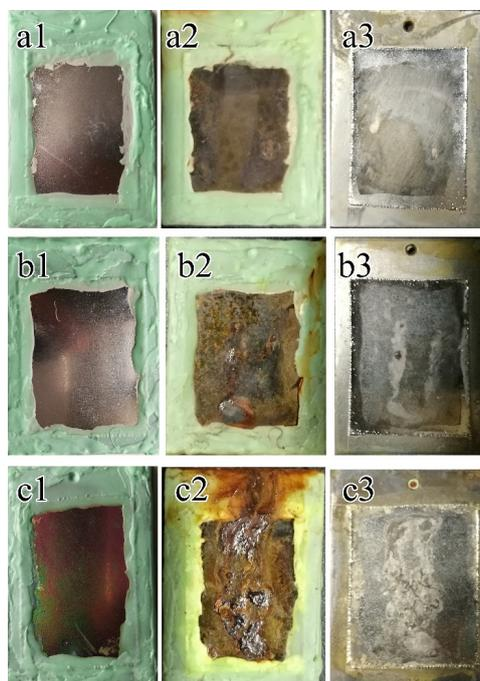
**Figure 8.** Corrosion results of samples deposited under SP. (a1) as deposited; (a2) as deposited after 1000 h test; (a3) as deposited with corrosion product removed; (b1) 300 °C treated; (b2) 300 °C treated after 1000 h test; (b3) 300 °C treated with corrosion product removed; (c1) 400 °C treated; (c2) 400 °C treated after 1000 h test; (c3) 400 °C treated with corrosion product removed.
