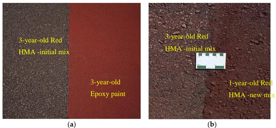
**Figure 9.** Visualization of tested surfaces: (a) Red HMA-initial mix and epoxy paint; (b) Red HMA-initial mix and Red HMA-new mix.
