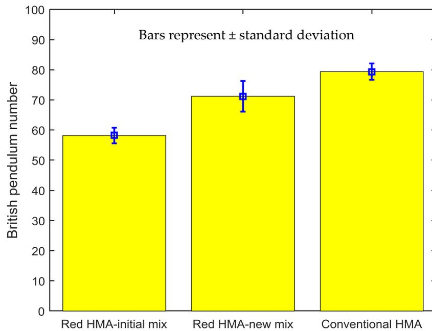
Figure 4. Pavement frictional values of tested sections.
