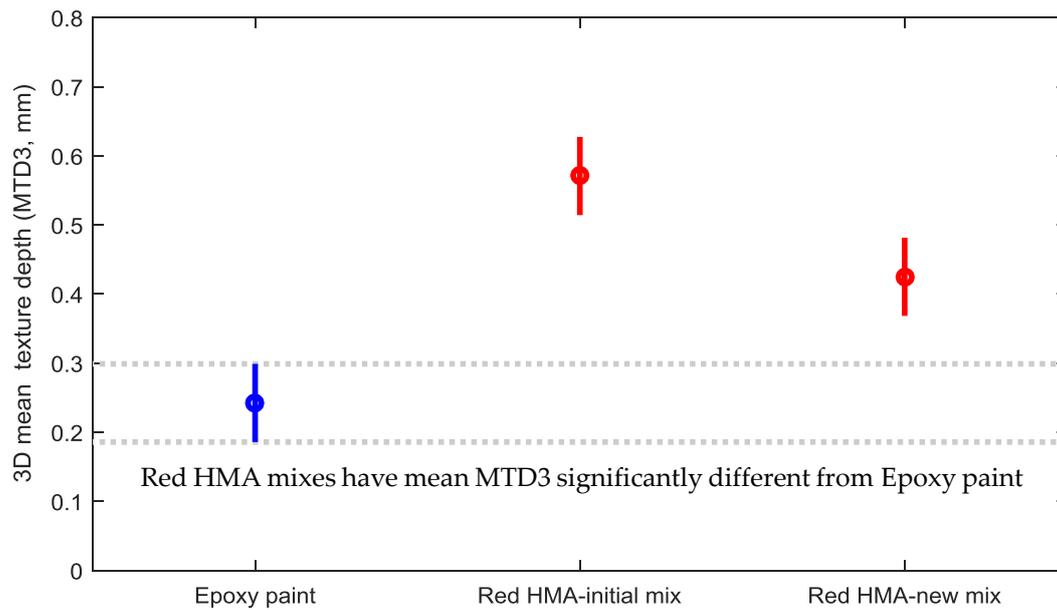
Figure 6. Pavement 3D mean macrotexture depths of tested sections.
