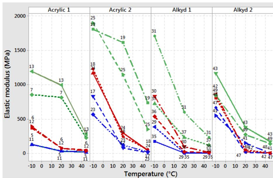
**Figure 4.** Influence of coating formulation on elastic modulus for the three test temperatures (in blue: clear PVC; in red: low PVC; in green: high PVC).
