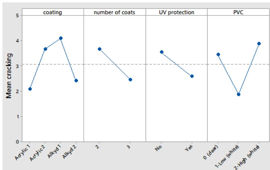
Figure 7. Main effects plot for the mean cracking.
