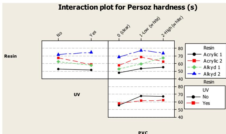
Figure 2. Interaction plot for the mean Persoz hardness.
