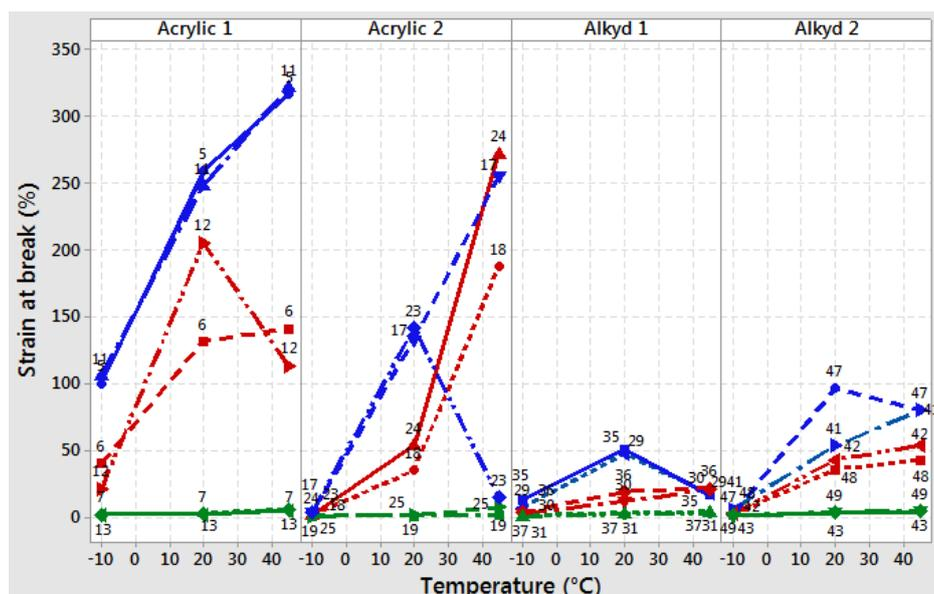
**Figure 5.** Influence of coating formulation on strain at break for the three test temperatures (in blue: clear PVC; in red: low PVC; in green: high PVC).
