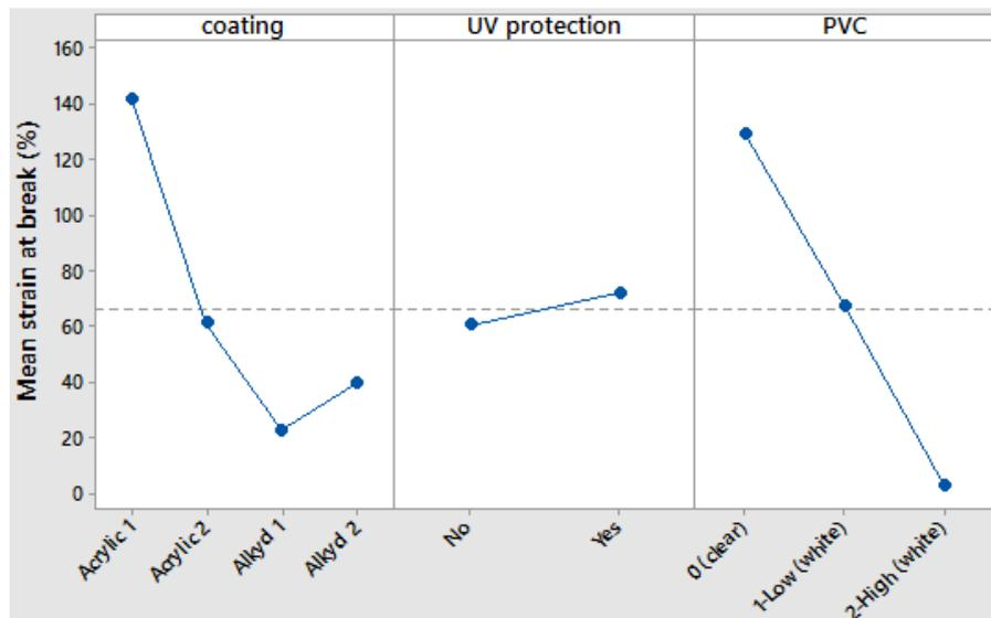
Figure 9. Main effects plot for the mean strain at break (room temperature).
