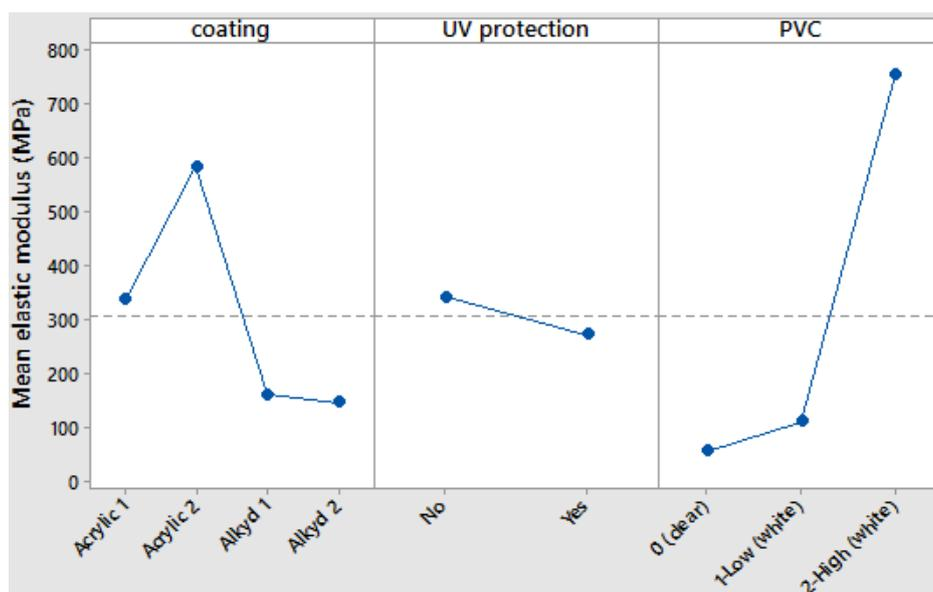
Figure 8. Main effects plot for the mean elastic modulus (room temperature).
