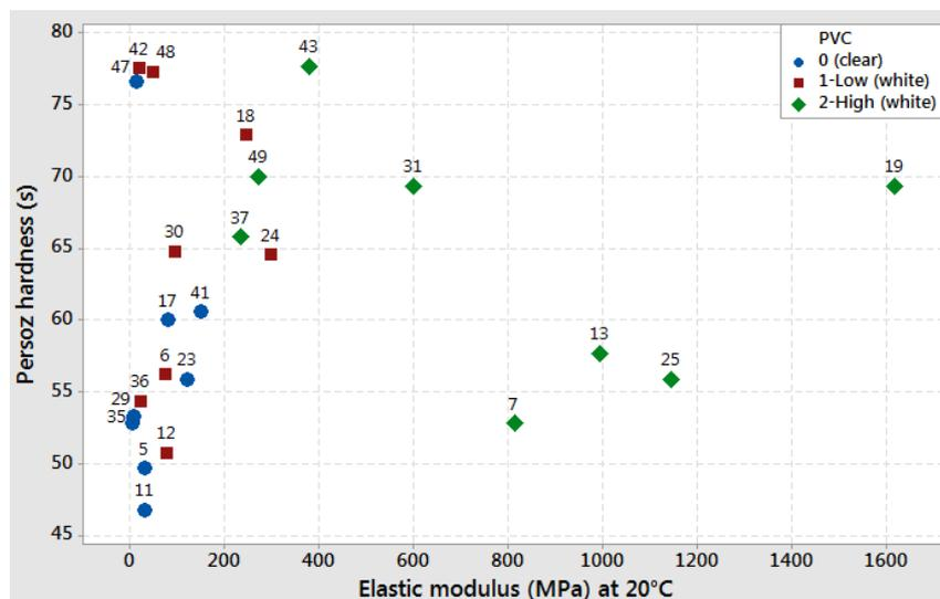
Figure 10. Relation between Persoz hardness and elastic modulus at room temperature.
