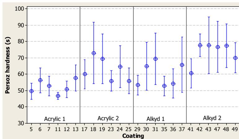
Figure 1. Mean Persoz hardness and confidence interval at 95% for the mean for the 24 coatings.
