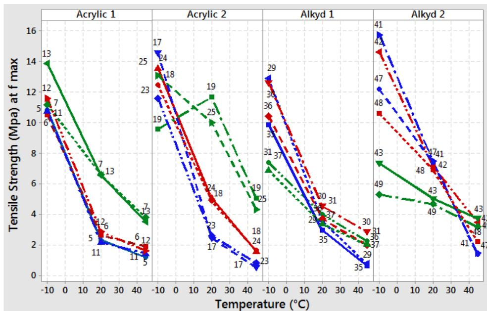
**Figure 6.** Influence of coating formulation on tensile strength for the three test temperatures (in blue: clear PVC; in red: low PVC; in green: high PVC).
