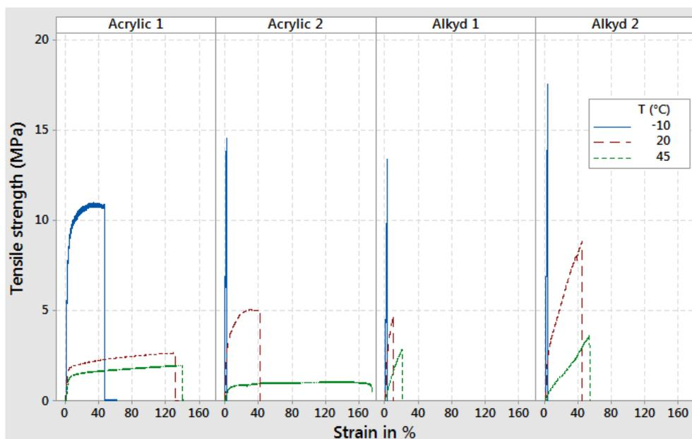
**Figure 3.** Comparison of the tensile strength–strain curves of the different coatings (examples with coatings 06, 18, 30, and 42 made with low PVC).
