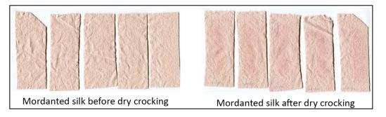
Figure 8. Mordanted silk dyed with draconin red before and after crocking.
