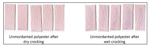
Figure 7. Unmordanted polyester dyed with draconin red shown after dry and wet crocking.
