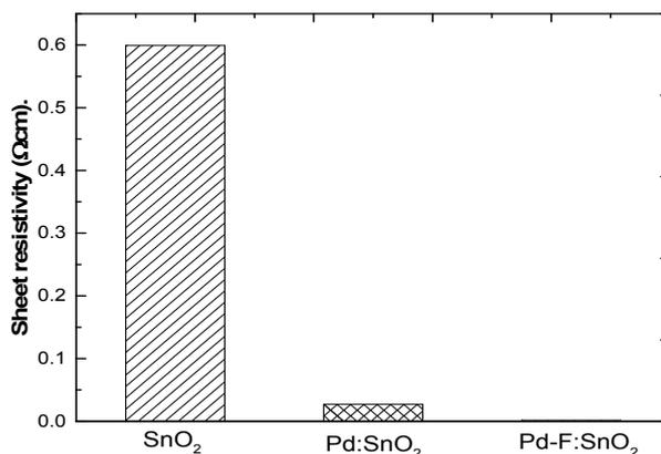
From Figure 6, the sheet resistivity of SnO<sub>2</sub> thin film decreases significantly when SnO<sub>2</sub> is doped with palladium at optimum condition (2.7 at% Pd) from  $5.992 \times 10^{-1} \Omega \text{ cm}$  to  $2.71 \times 10^{-2} \Omega \text{ cm}$ . A similar decrease is observed when fluorine is added to Pd:SnO<sub>2</sub>, the resistivity decreases from  $2.71 \times 10^{-2}$  to  $1.64 \times 10^{-4} \Omega \text{ cm}$  for 16.04 at% F.
