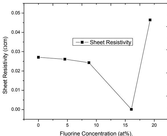
The Pd-F:SnO<sub>2</sub> thin films with the least sheet resistivity was obtained at 16.04 at% F. Upon increasing the dopant concentration above the optimum level of doping, the sheet resistivity increased again. This is attributed to deterioration of the crystal structure hence decreasing the mobility of the free electrons which lead to an increase in the sheet resistivity of the thin films [20].
