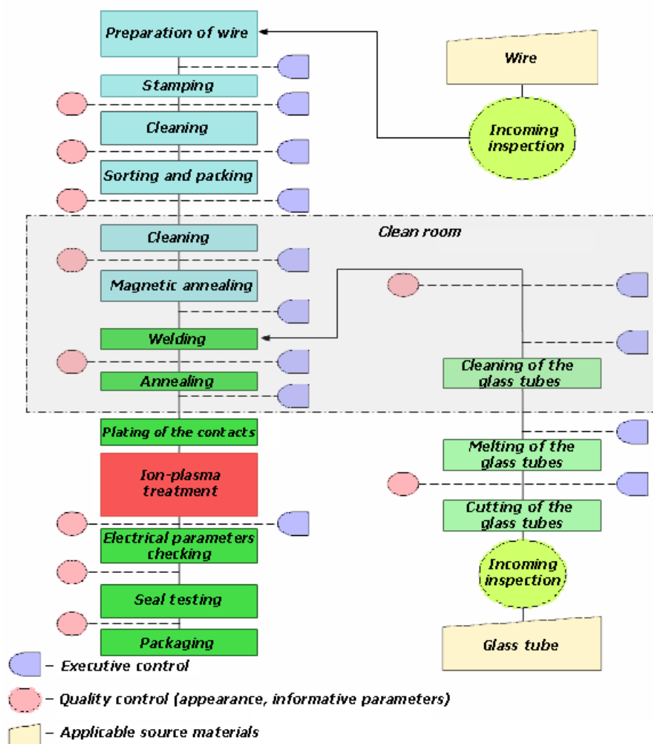
Figure 2. The manufacturing route of MKA-14108 production.
