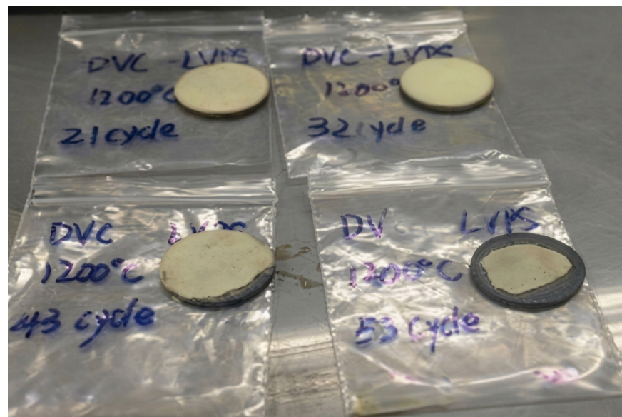
Figure 13. Interfacial delamination morphologies of the specimens subjected to varying thermal cycles.
