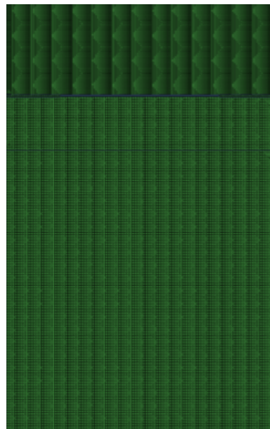
Figure 18. Schematic of the finite element simulation model for TBC ultrasonic propagation.
