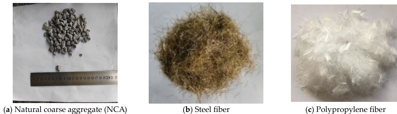
Figure 1. Coarse aggregate and fiber.
