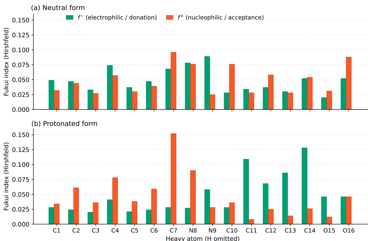
Figure 10. Condensed Fukui indices ( f^+ and f^- ) illustrating the (a) neutral and (b) protonated states of FNH.
