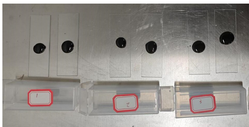
Figure 8. AFM test samples of three types of asphalt mastic.
