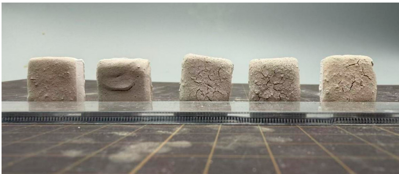
Figure 11. Images of G1 through G5 being fired at 1100 degrees Celsius.
