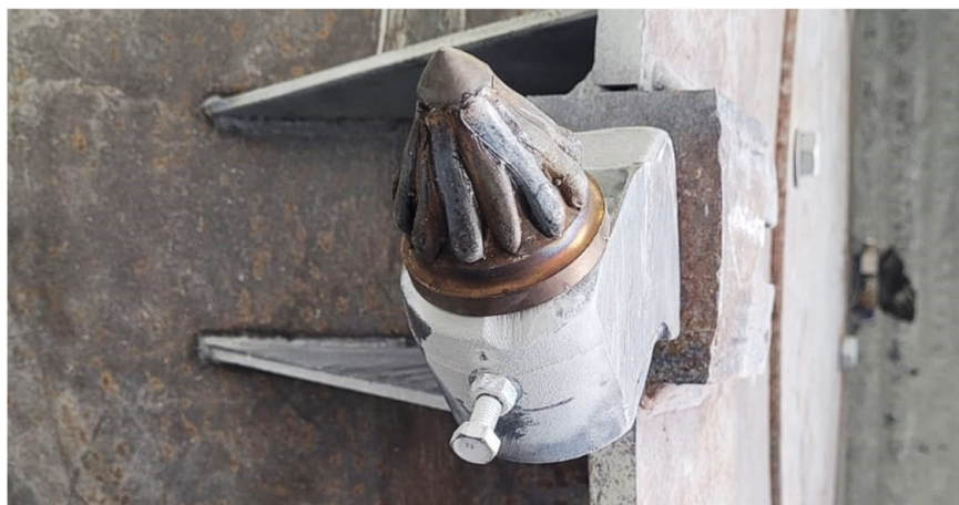
Figure 1. Exemplary picture of a mining cutting tool with hard-faced wear-resistant overlay fabricated with one of the studied materials.
