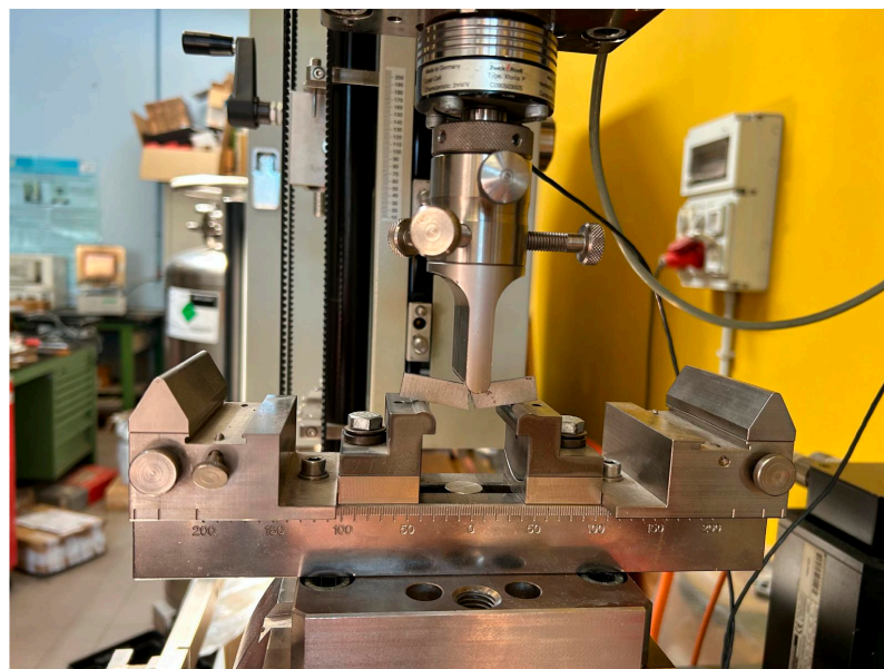
Figure 5. The TRS test with the BPEI/SiO 2 SMC sample under examination.
