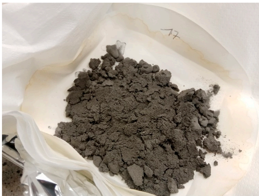
Figure 3. Coated iron powder after the drying phase.
