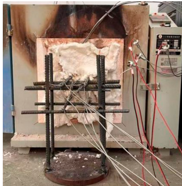
Figure 5. Apparatus for thermal insulation test.
