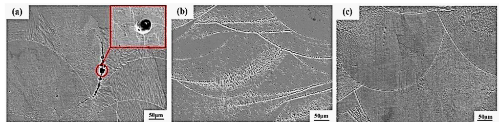
Figure 11. SEM images of the composite samples with different laser powers: (a) P = 160 W, (b) P = 180 W, (c) P = 200 W.
