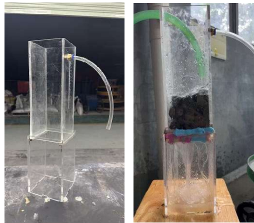
Figure 4. Photos showing the horizontal permeability testing device and experimental process.
