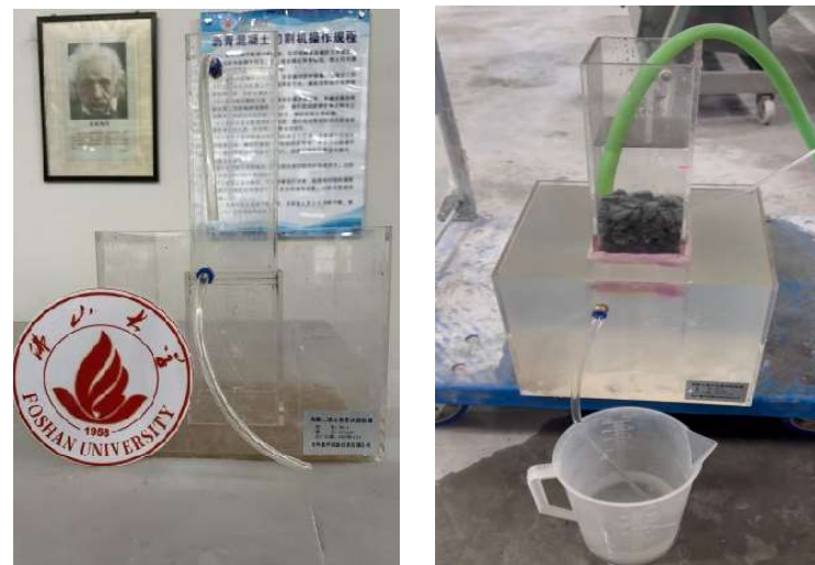
Figure 3. Photos showing the vertical permeability testing device and experimental process.
