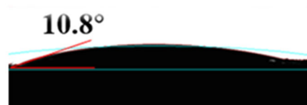
Figure 14. Water contact angle of PFC after 25 freeze–thaw cycles.
