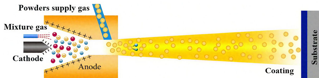
Figure 10. Schematic diagram of plasma spray [61].
