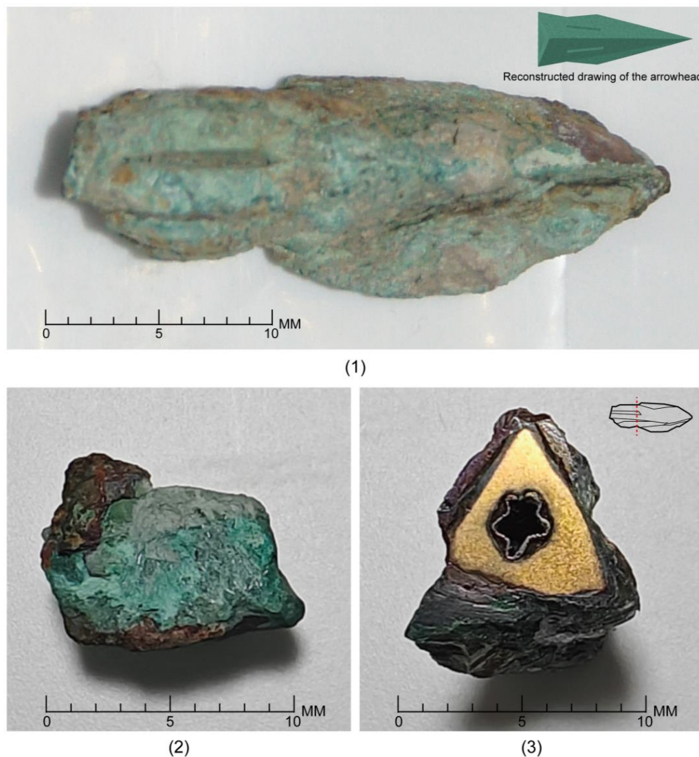
Figure 4. Detailed illustration of the samples used in this study. (1) Intact bronze arrowhead sample. (2) Image of copper rust on the arrowhead surface. (3) Cross-sectional image of the arrowhead (image source: photographed and annotated by the author).
