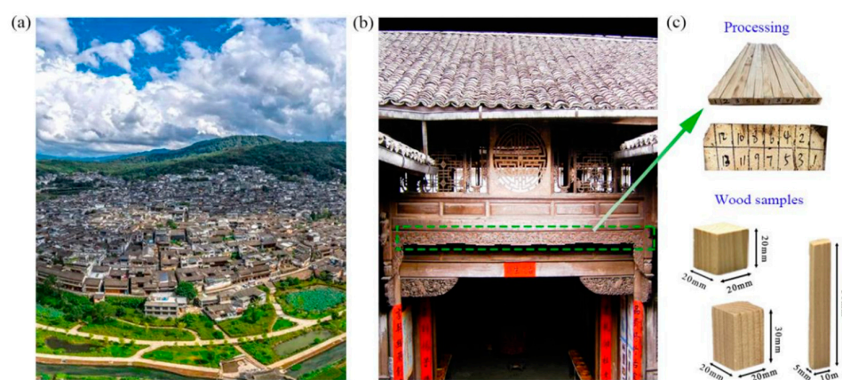
Figure 1. (a) The overlooking view of the ancient town. (b) Location of collected wood components. (c) Wood component processing and test samples; the test includes surface composition, wettability characterization, and water uptake/moisture absorption measurement [1].
