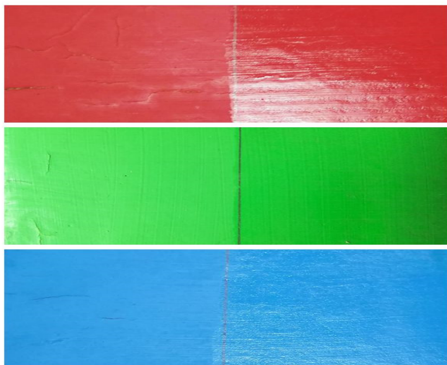
Figure 7. Photographs of red, green, and blue painted wood plates after 20 days accelerated aging in UV weathering chamber.
