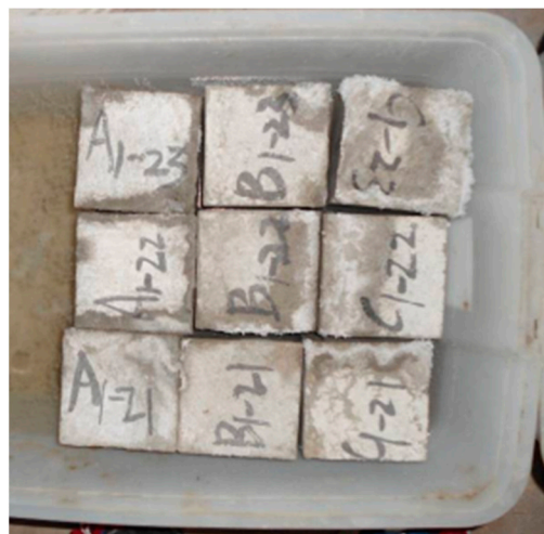
Figure 8. The specimen was soaked in a sodium sulfate solution.
