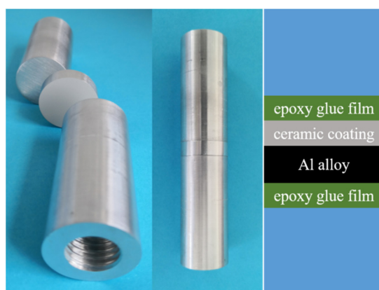
Figure 2. Illustration of the direct pull-off tensile test.
