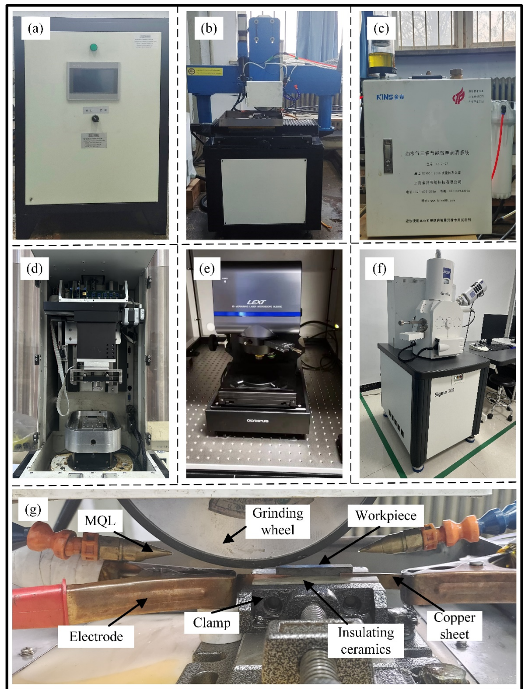
Figure 1. Laboratory equipment. (a) Pulsed power supply, (b) grinder, (c) minimal quantity lubrication device, (d) friction and wear tester, (e) OLS5000 confocal laser scanning microscope (Japan), (f) Sigma300 field emission scanning electron microscope, (Sigma, Taufkirchen, Germany), (g) power-up method.
